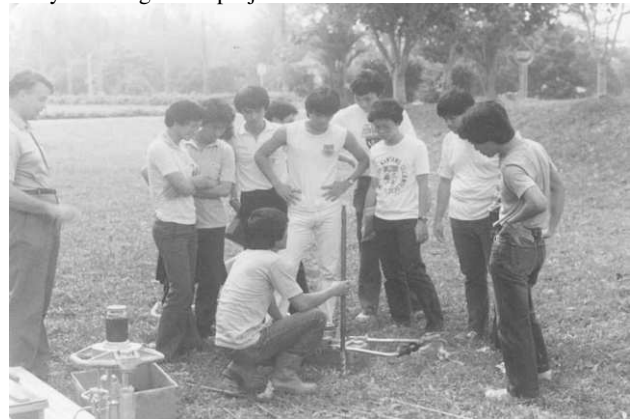
Prof. Bengt Broms with NTI students learning about the Weight Sounding test, routinely used in Sweden.
