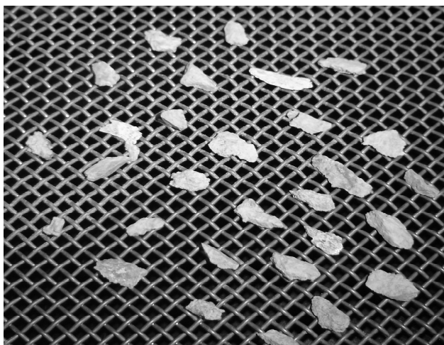
(b) Material coarser than 4.75 mm in the investigated waste rock
