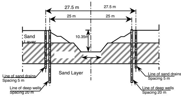
Figure 5. Excavation configuration required for construction of the typical culvert sectors.
