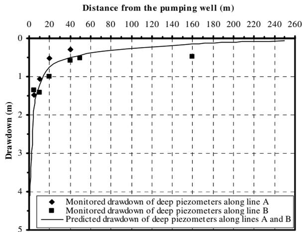
Figure 2. Comparison of monitored and predicted drawdown values within the bottom sand aquifer, pumping test (1).
