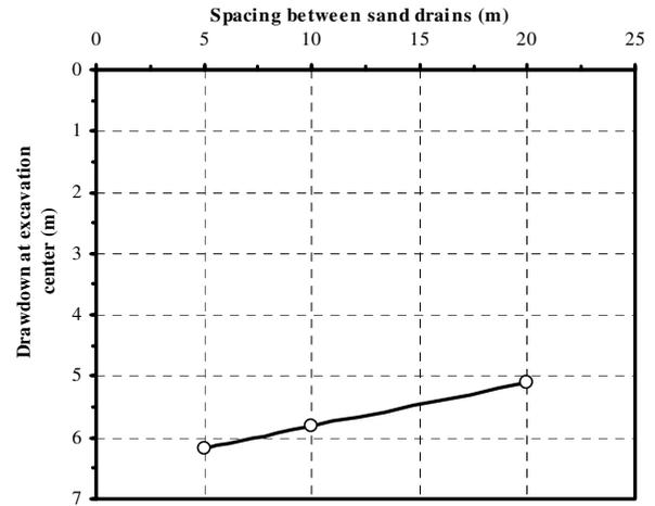
Figure 7. Effect of sand drains spacing on the drawdown at excavation center
