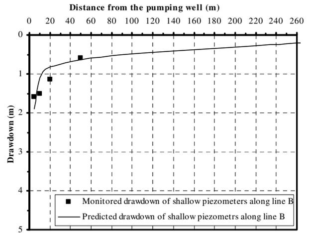
Figure 4. Comparison of monitored and predicted drawdown values within the top sand aquifer, pumping test (2).
