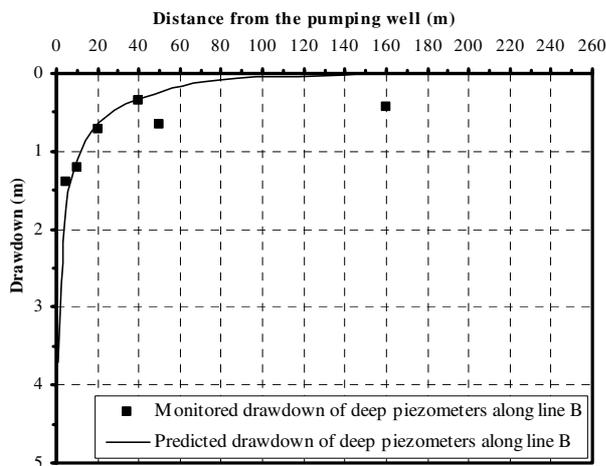
Figure 3. Comparison of monitored and predicted drawdown values within the bottom sand aquifer, pumping test (2).
