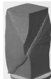
Photo 1. Picture of shear bands after CIU test and breaching of river embankment due to heavy rains.
