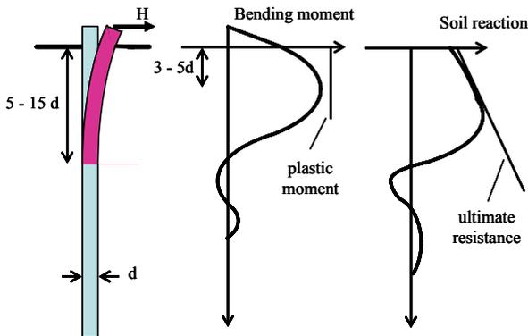
Figure 3.17 Schematic of laterally loaded pile response
