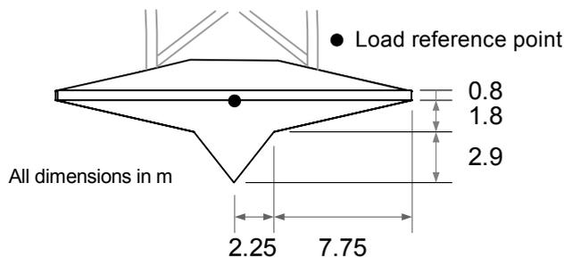
Figure 5.27 Assumed spudcan shape in numerical examples
