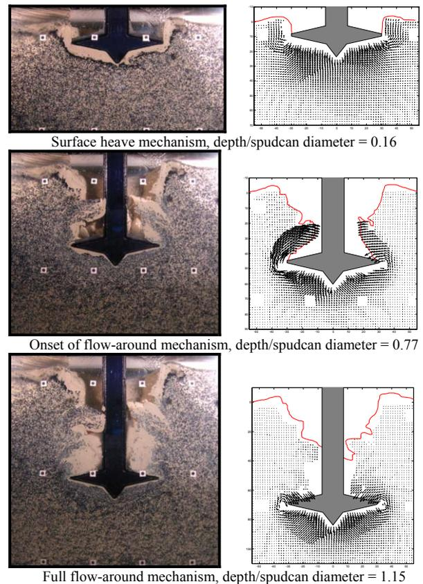
Figure 5.8 Digital images and PIV analysis of flow vectors from centrifuge tests (after Hossain et al., 2004)
