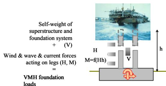
Figure 4.2 Combined loading of a gravity base platform
