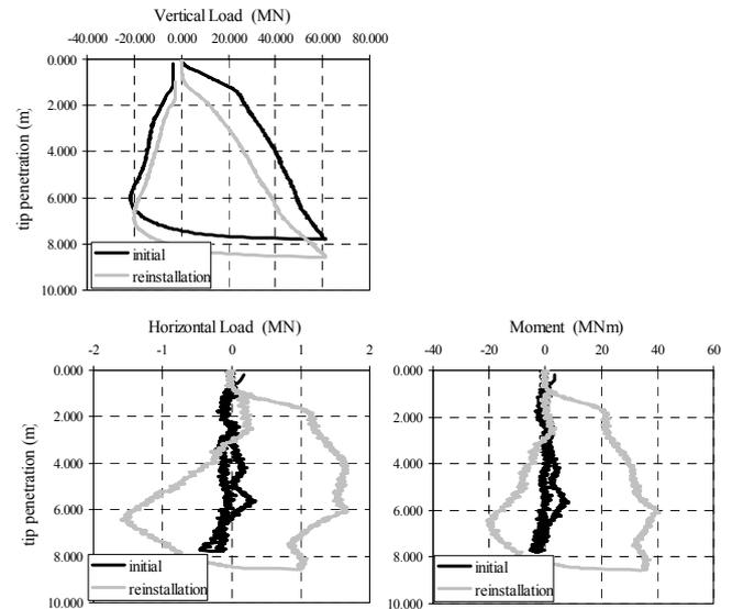
Figure 5.15 Measure combined loads on spudcan during reinstallation experiment (in scaled prototype units)
