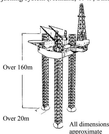
Figure 5.1 Typical jack-up unit used today (after Reardon, 1986)
