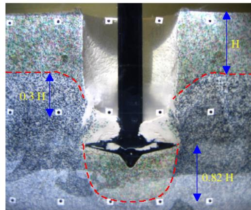
Figure 5.12 Captured image of a penetrating half-spudcan in two-layered clay (after Hossain et al., 2005)
