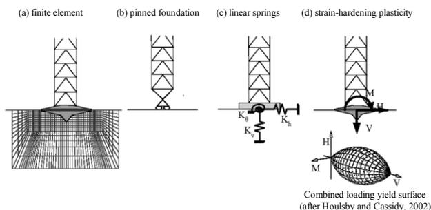
Figure 5.17 Spudcan – soil interaction analysis methods
