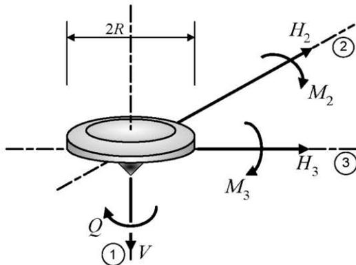
Figure 5.4 Combined loads on a spudcan footing
