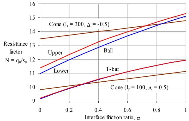
Figure 2.6 Theoretical factors for cone, T-bar and ball
