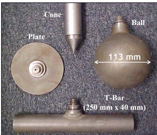
Figure 2.5 Alternative full-flow penetrometers with cone
