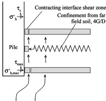
Figure 3.5 Schematic for friction fatigue (White & Bolton, 2004)
