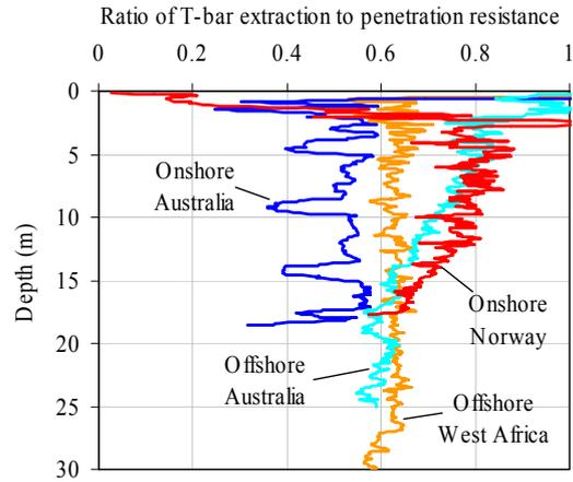
Figure 2.8 Ratio of extraction to penetration resistance for T-bar
