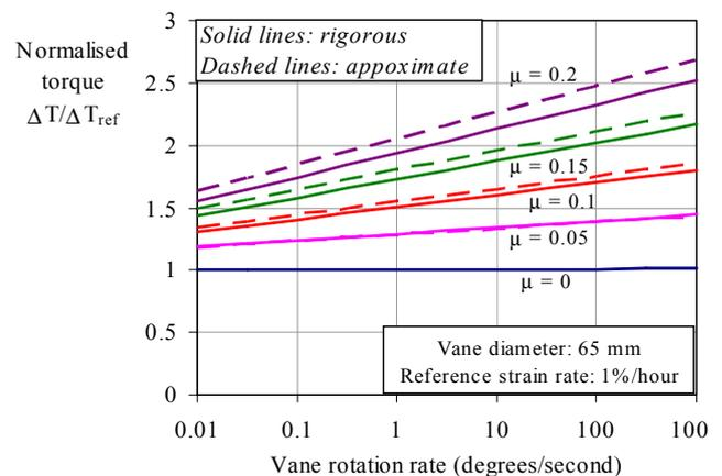
Figure 2.4 Effect of vane rotation rate on torque
