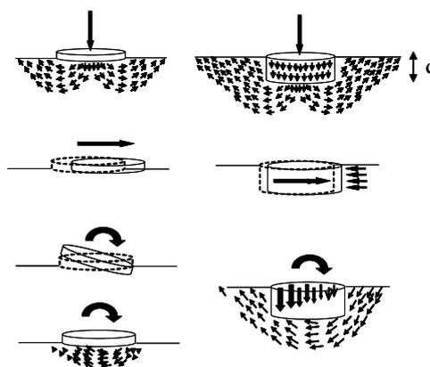
Figure 4.16 Enhanced foundation capacity due to embedment
