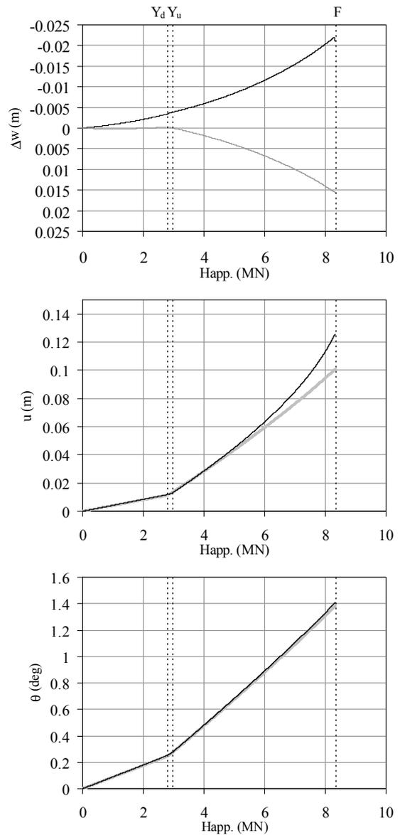
Figure 5.28 Load and displacement paths followed by spudcans during quasi-static pushover.
