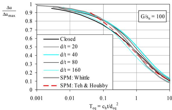
Figure 3.10 Pore pressure dissipation at pile shaft (Randolph, 2003)
