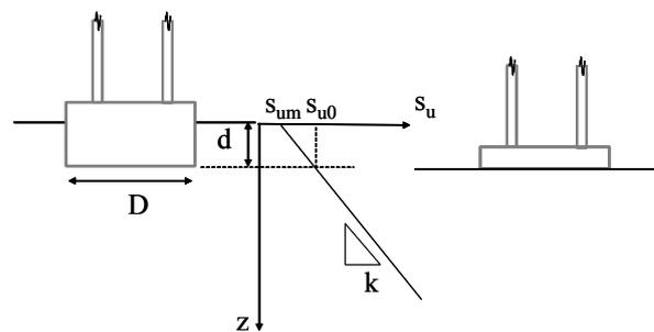
Figure 4.13 Conceptual modelling of foundation skirts in numerical analyses
