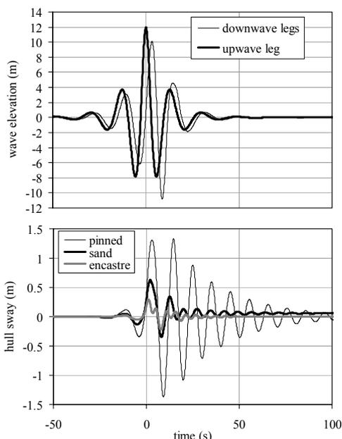
Figure 5.31 Horizontal hull movement during wave loading event
