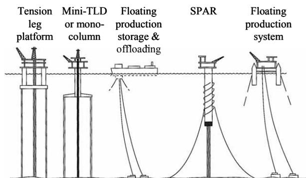
Figure 6.1 Floating system options (Leffler et al., 2003)
