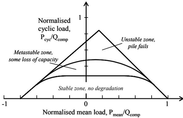
Figure 3.12 Cyclic stability diagram (after Poulos, 1988)
