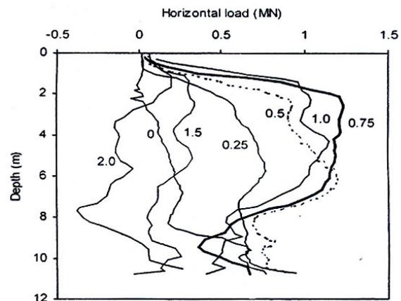
Figure 5.16 Measured horizontal loads at offset distances (expressed as a multiple of spudcan diameter) (after Stewart & Finnie, 2001)
