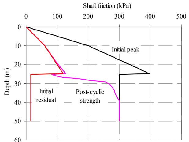
Figure 3.14 Profiles of peak, residual and post-cyclic shaft friction
