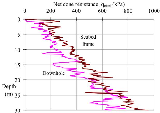
Figure 2.2 Comparison of downhole and seabed frame CPTs
