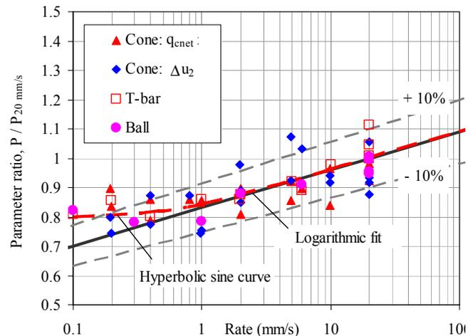
Figure 2.13 Effect of penetration rate for undrained conditions
