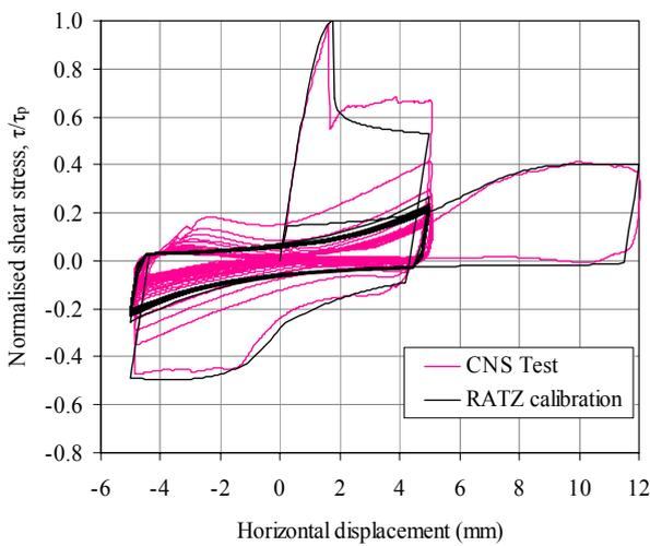
Figure 3.13a Calibration of RATZ against CNS test data
