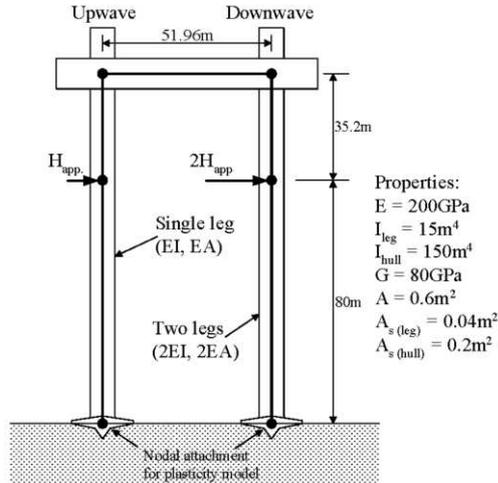
Figure 5.26 Jack-up model and loading for pushover analysis
