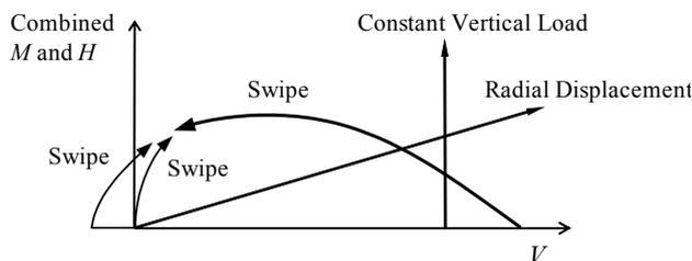
Figure 5.20 Experimental load paths followed to develop strain-hardening plasticity models
