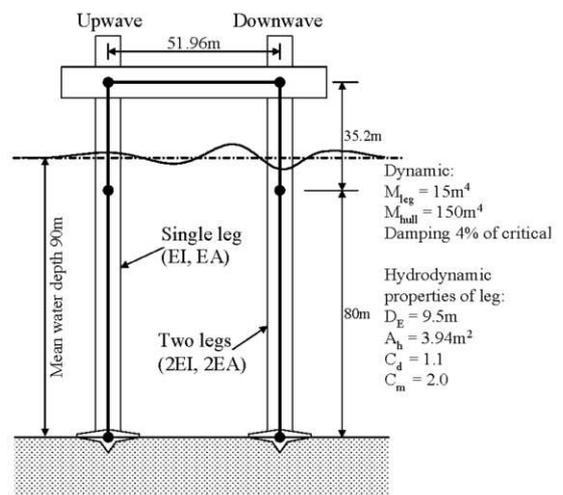
Figure 5.30 Properties used in dynamic environmental loading example
