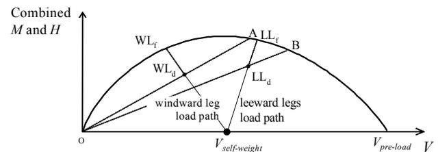
Figure 5.5 Expected load paths during a typical site-assessment
