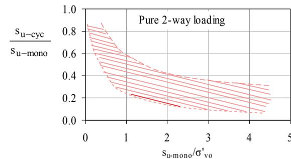
Figure 2.16 Cyclic strength database for uncemented carbonate soils.
