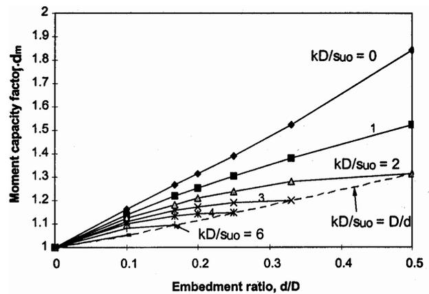
Figure 4.18 Upper bound prediction of moment capacity factor with embedment (Bransby & Randolph, 1999)
