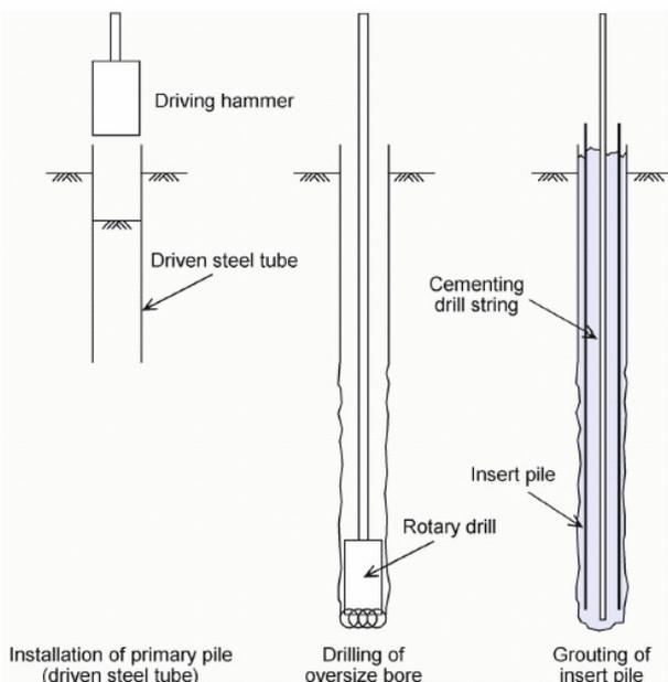
Figure 3.2 Stages in installation of an offshore drilled and grouted pile
