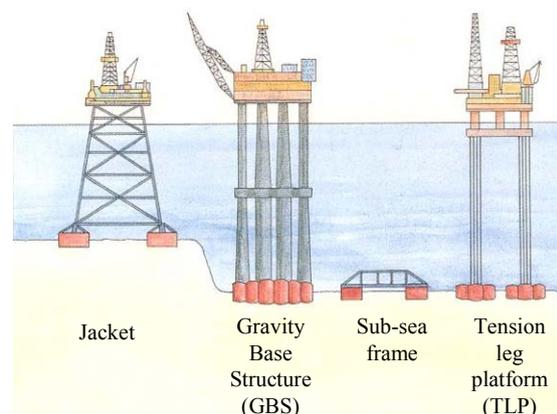
Figure 4.1 Applications of offshore shallow foundations (NGI)
