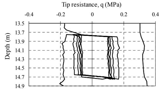
Figure 2.9 Cyclic T-bar test at depth 14.3 m (Chung & Randolph, 2004)
