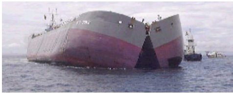
Figure 18. Soil dumping by hopper barge
