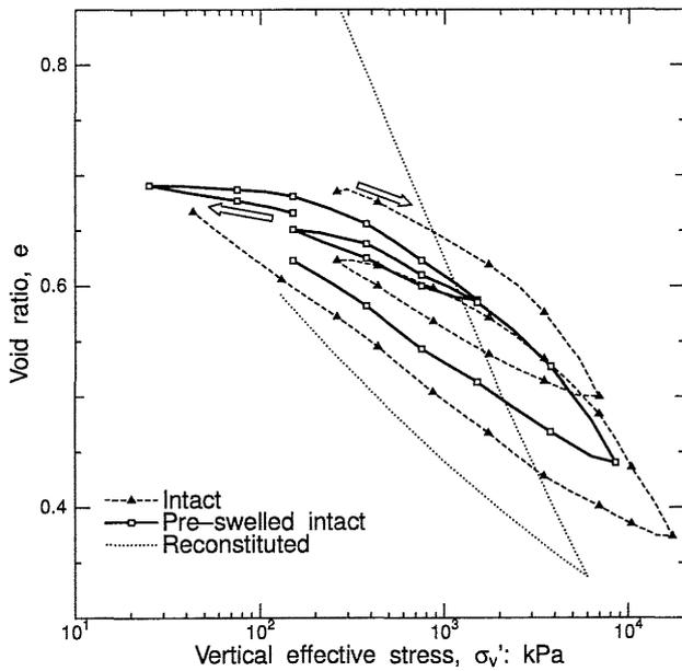
Figure 4. Volume change in one-dimensional compression and unloading (Ma, 2003).
