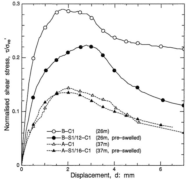
Figure 6. Normalised shear stress–horizontal displacement relations ( $\sigma'_{v0} = 300$  &  $400$  kPa).
