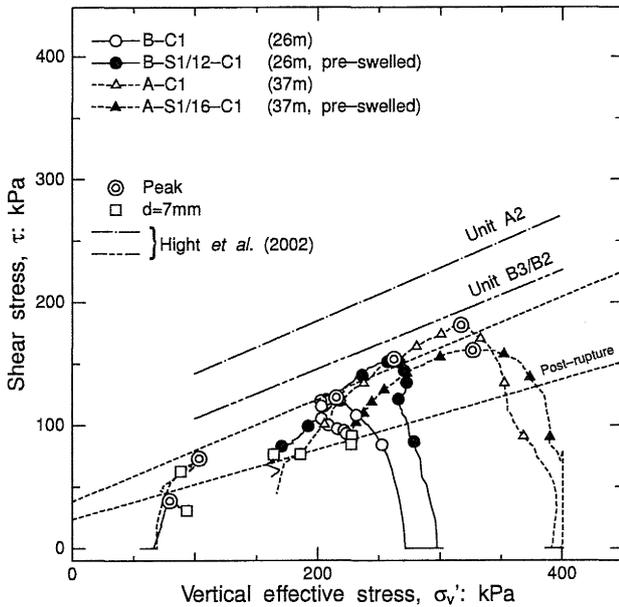
Figure 5. Stress paths in constant-height direct shear box test ( $\sigma'_{v0} \leq 400$  kPa).
