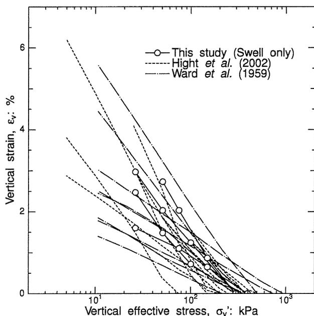
Figure 2. Vertical strain changes in one-dimensional swelling tests.
