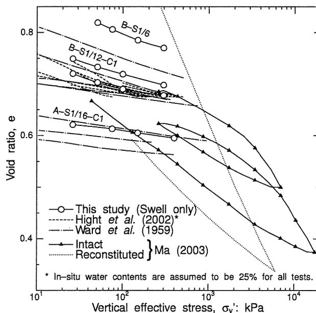
Figure 3. Volume change in one-dimensional swelling together with those in compression and unloading curves on intact and reconstituted samples.
