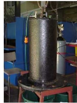
Figure 3. Porous brick pressure testing chamber
