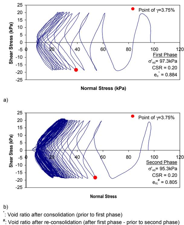
Figure 3. Stress path observed during constant volume cyclic DSS loading of Fraser River Silt. a) First cyclic loading phase, b) Second cyclic loading phase.
