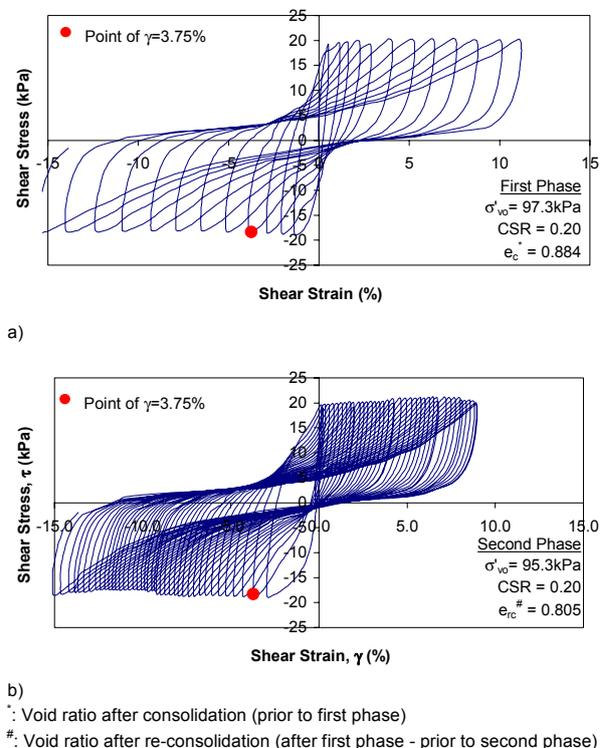
Figure 2. Stress strain response during constant volume cyclic DSS loading of Fraser River Silt. a) First cyclic loading phase, b) Second cyclic loading phase.
