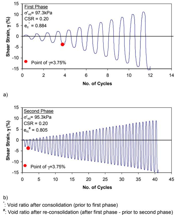
Figure 5. Shear strain development with the number of cycles during constant volume cyclic DSS loading of Fraser River Silt. a) First cyclic loading phase, b) Second cyclic loading phase.
