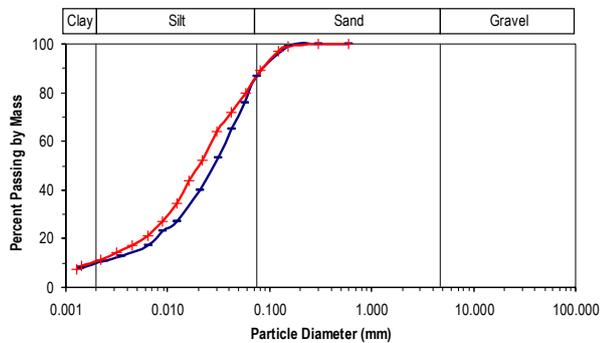
Figure 1. Grain size analysis from two representative soil samples of Fraser River Delta silt.
