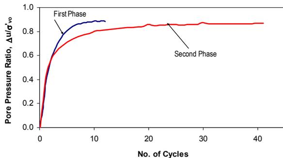
Figure 4. Maximum pore water pressure ratio vs. number of cycles during constant volume direct simple shear test on Fraser River Delta silt.
