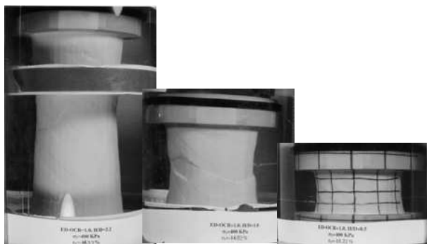
Figure 1. Comparison of necking in clay specimens with H/D ratios of 2.2, 1.0 and 0.5 at approximately 15% axial strain
