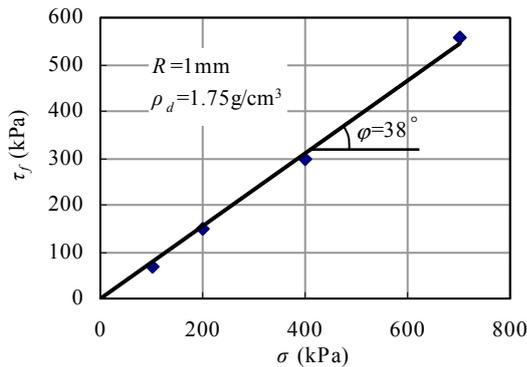
Fig.3 Shear strength of the interface between steel plate and gravel
