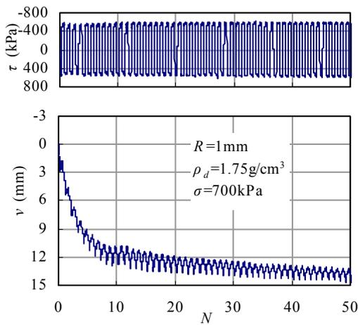
Fig.4 Cyclic history under constant normal stress boundary condition
