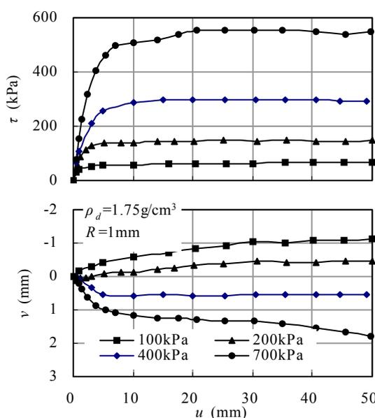
Fig.2 Monotonic test results under constant normal stress boundary condition
