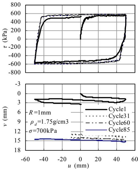
Fig.5 Cyclic stress-displacement relationship under constant normal stress boundary condition
