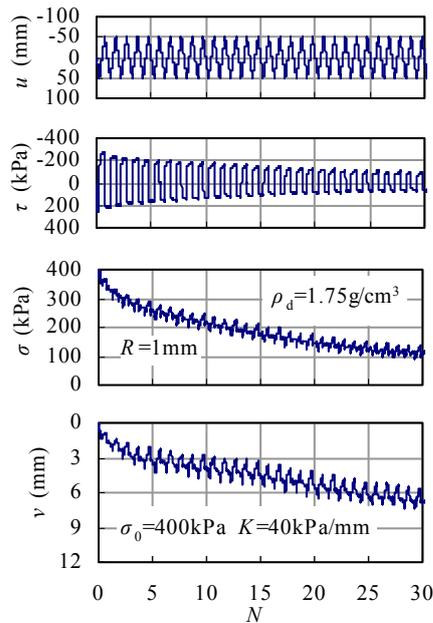
Fig.6 Cyclic history under constant normal stiffness boundary condition
