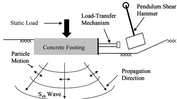
Figure 3. Generation of linear and nonlinear  $S_{vh}$  waves using a pendulum hammer
