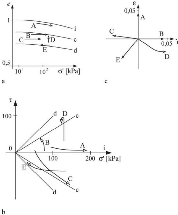
Fig. 4 Evolution of void ratios (a), stresses (b) and strains (c) towards state limits
