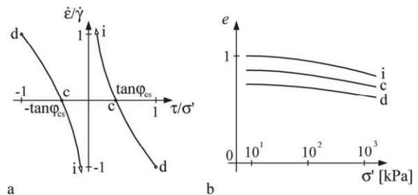
Fig. 2 Strain rate ratio vs. stress ratio (a) and void ratio vs. pressure (b) for state limits of psammoids
