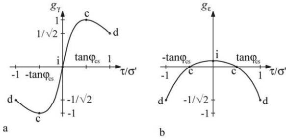
Fig. 3 Factors for plastic strain rates
