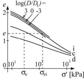
Fig. 5 Isotachs of void ratio vs. effective pressure for a peloid
