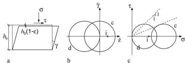
Fig. 1 Simple shearing (a), Mohr diagrams of strain rates (b) and stresses (c) for state limits
