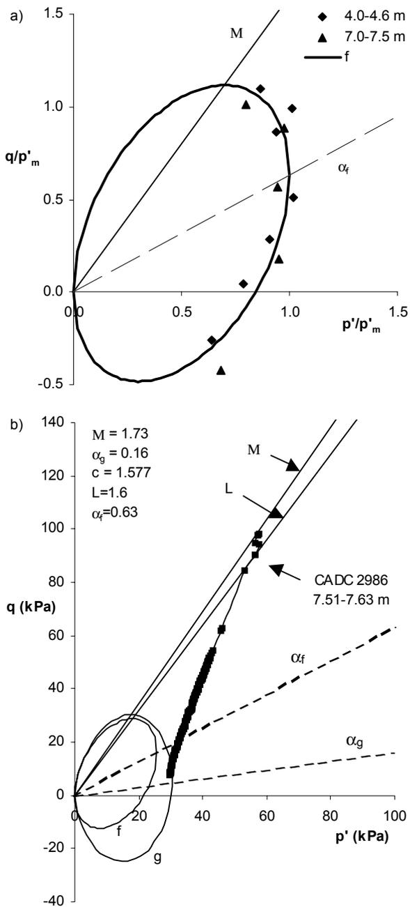
Figure 1. a) Yield curve for natural Murro clay. b) Yield curve, plastic potential and the stress path of the drained test CADC 2986 on natural Murro clay.
