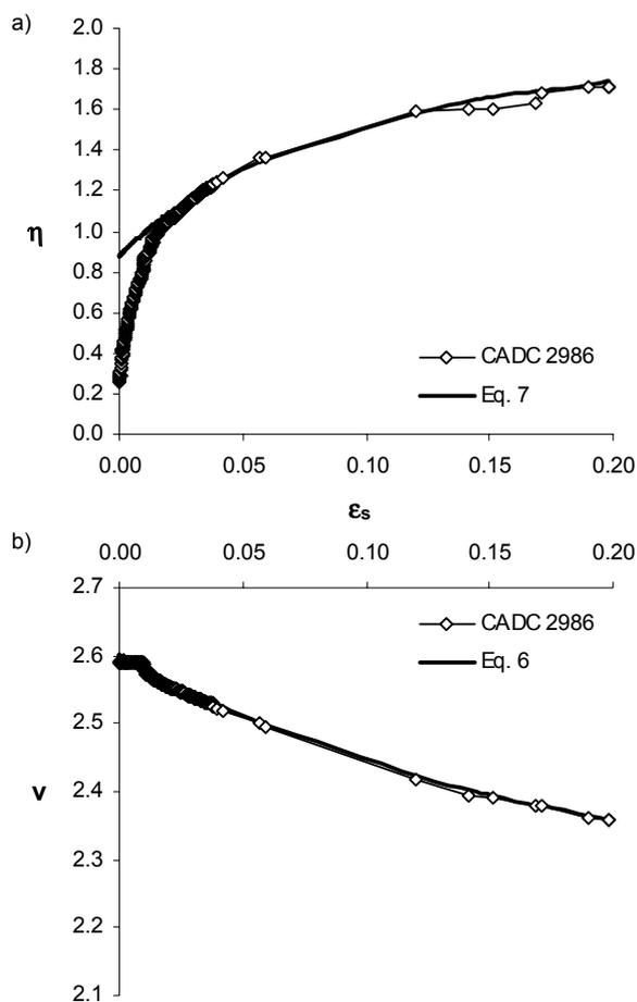
Figure 2. Results of test CADC 2986 on Murro clay from the depth of 7.51-7.63 m and calculations with the deformation equations.
