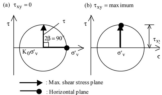
Figure 2. Swinging of the plane of maximum shear stress under  $K_0$  condition
