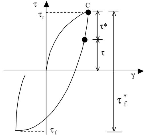
Figure 6. Stress ratio during unloading and reloading
