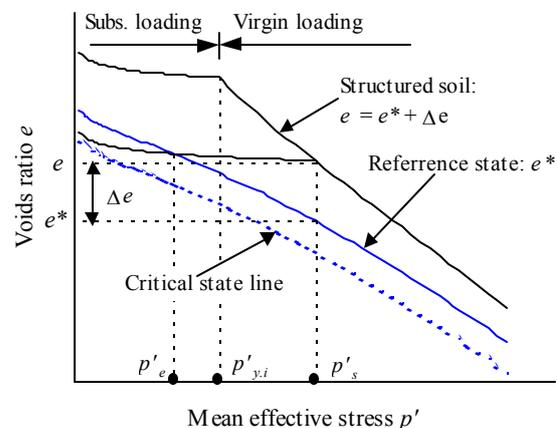
Figure 2 Compression behaviour of soil
