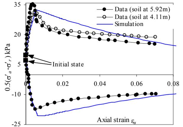
Figure 4 Stress-strain behaviour of Emmerstad clay
