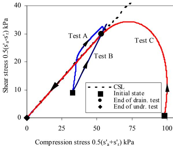
Figure 5 Simulated stress paths for Emmerstad clay in both drained and undrained tests
