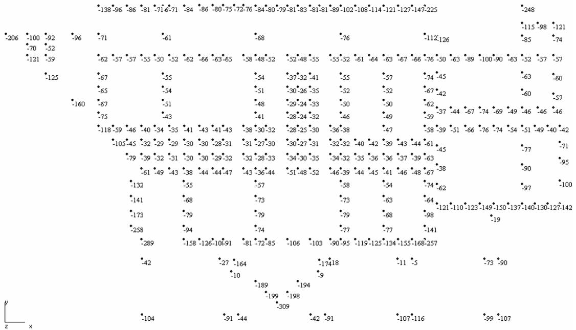
Figure 4. Loads on piles (tonne/force) under a building section
