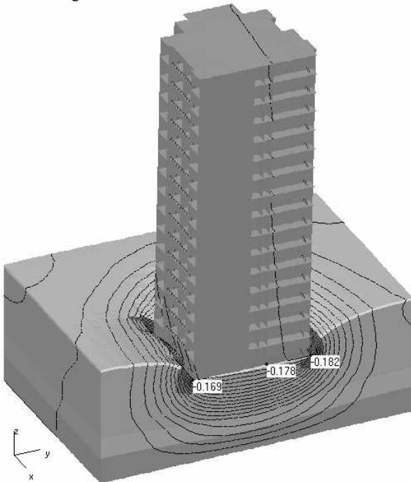
Figure 1. Deformation profile and isolines of settlement (m) of foundation and surrounding soil (cross-section). Shaded areas designate the zones of limiting state development in soil
