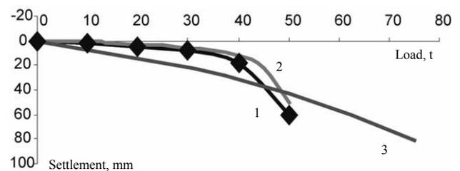
Figure 6. Load-settlement curve: 1 – pile displacement as per classical single static test; 2 – pile displacement as per calculation for a single static pile test model; 3 – pilecap settlement as per calculations
