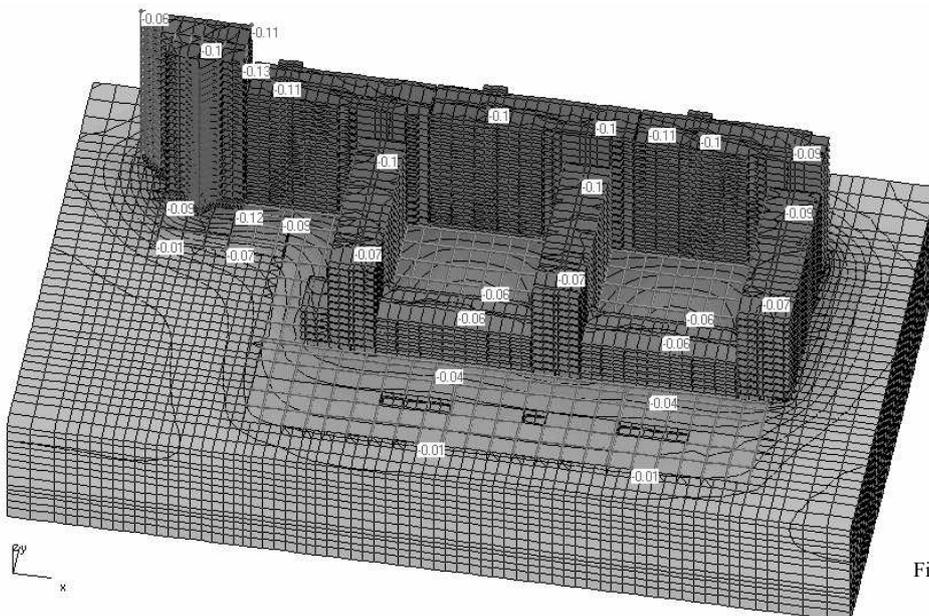
Figure 3. Isolines of vertical displacements (m)
