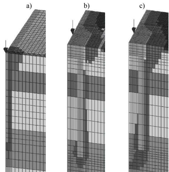
Figure 5. Zones of limit state development in soil (shaded): a – for a single pile test model; b, c – for a pile-cap interaction model. The load on pile is 50 t (a); 37.5 t (b) and 50 t (c)
