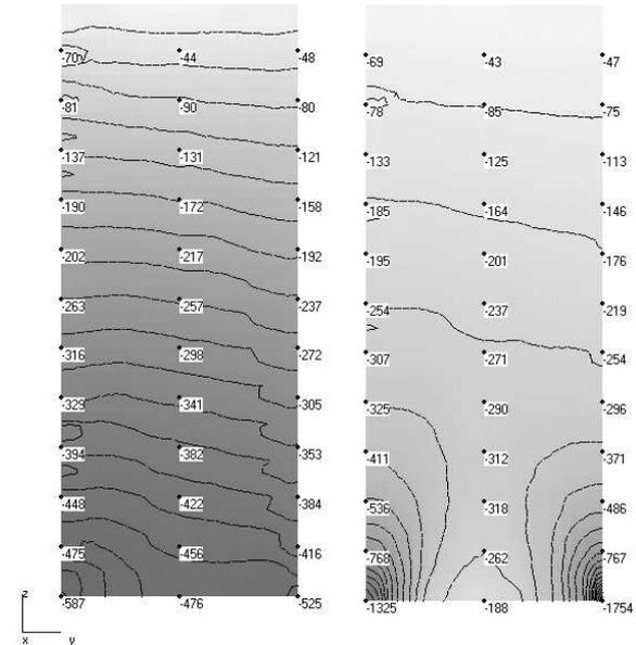
Figure 2. Isolines of vertical normal forces in the transverse wall: a - irrespective of soil-foundation deformability; b - according to soil-structure interaction calculations (kN/linear m)
