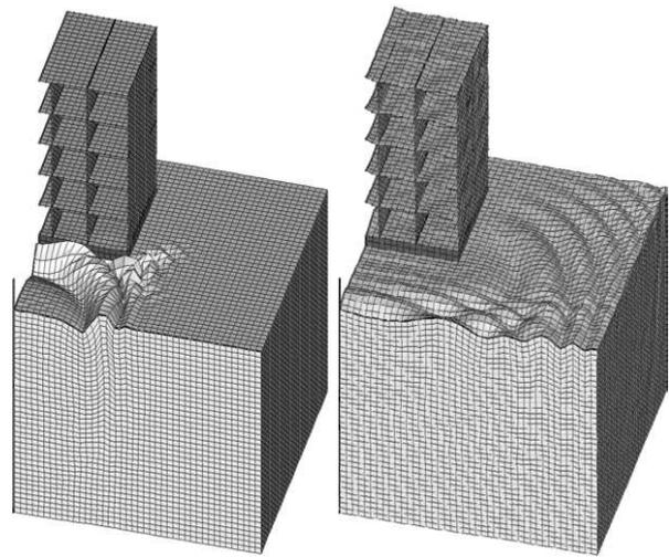
Fig. 7. Deformation profile. Waves propagation with account of interaction with superstructure at different time intervals
