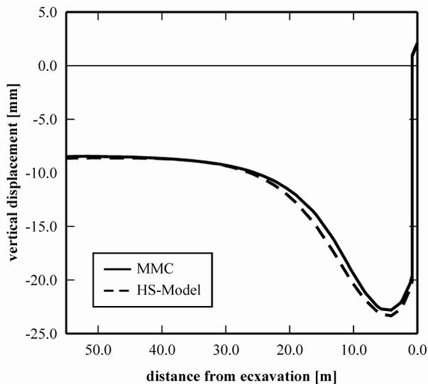
Figure 10. Settlements behind wall for project "AMV"
