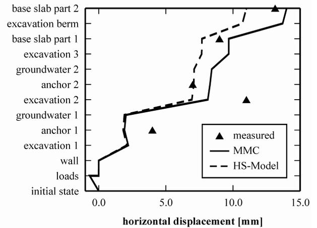
Figure 7. Horizontal displacement of wall head for project "Hypobank"
