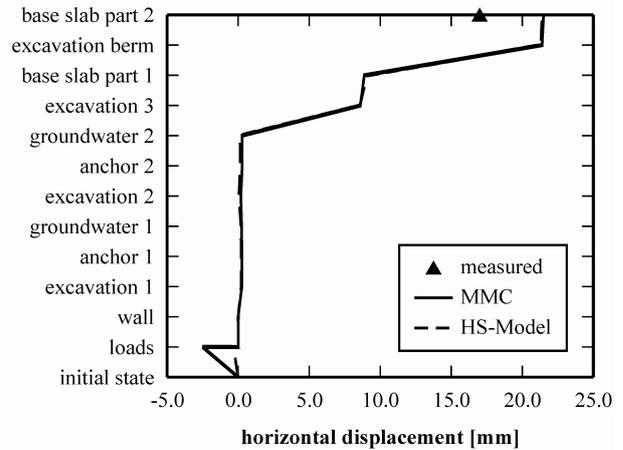
Figure 11. Horizontal displacement of wall head for project "AMV"
