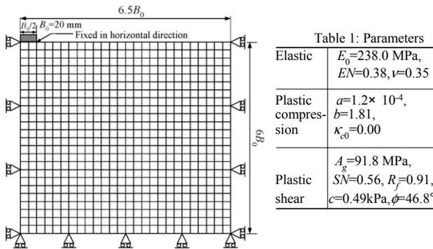
Figure 2. FE-mesh and boundary conditions.
