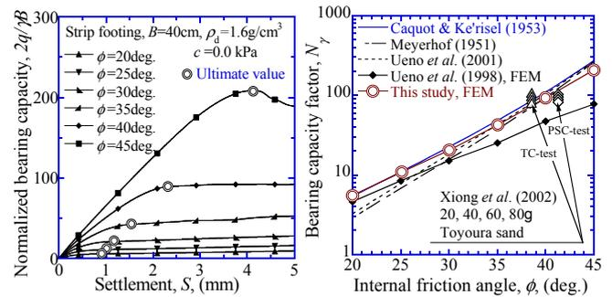
(a) Load-settlement relationships (b) Bearing capacity factor,  $N_\gamma$
