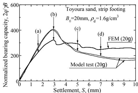
Figure 3. Relationships between normalized bearing capacity and footing settlement from FEM, compared with those from loading tests (20g).
