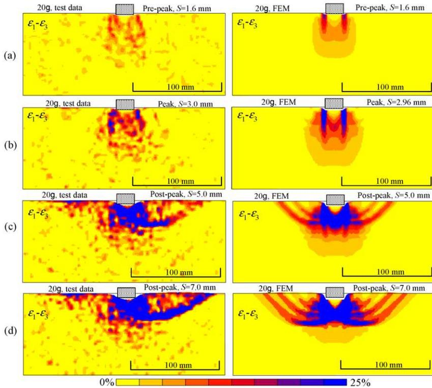
Figure 5. Measured and calculated maximum shear strain distribution for a 20g loading test on a dense Toyoura sand.
