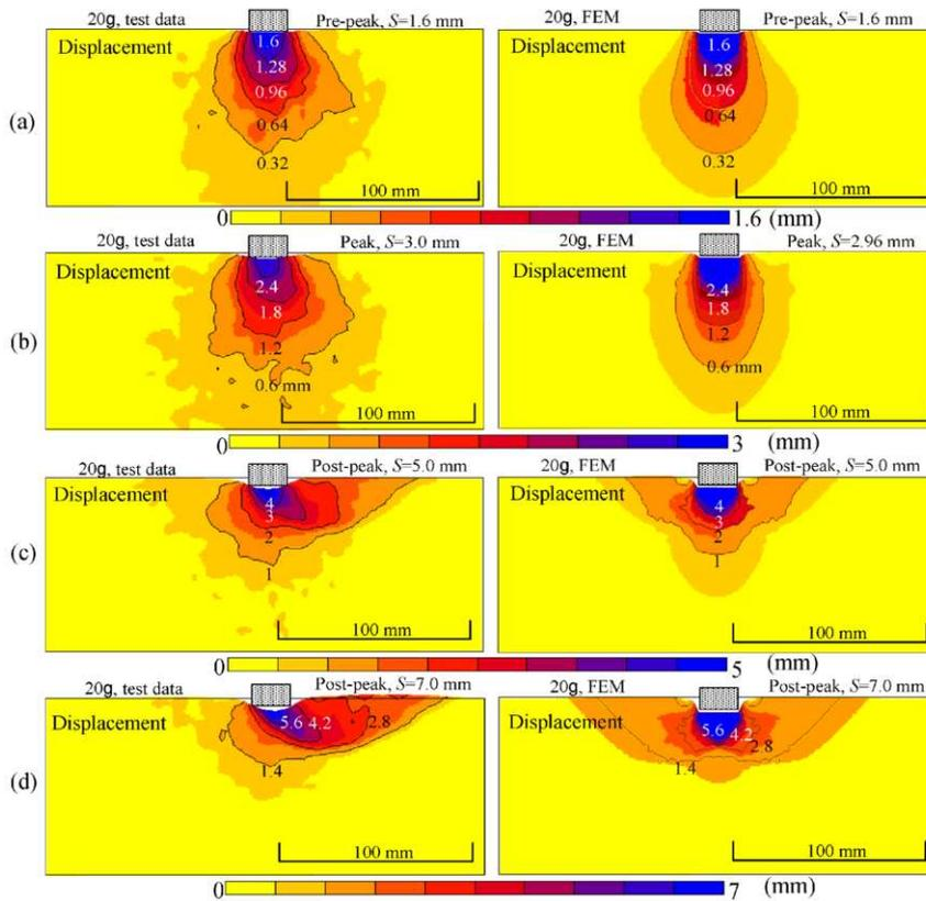
Figure 4. Measured and calculated displacement distribution for a 20g loading test on a dense Toyoura sand.
