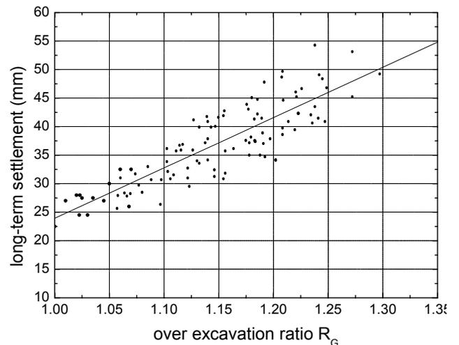
Fig.6 Correlation between long-term surface settlement and the over-excavation ratio(Lee, et al. 1999)
