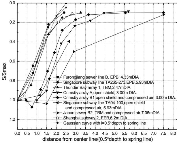
Fig.3 Long-term surface settlement troughs corresponding to different tunnel excavation methods
