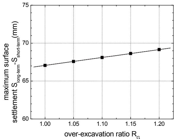
Fig.5 Development of post-construction surface settlement with over-excavation ratio
