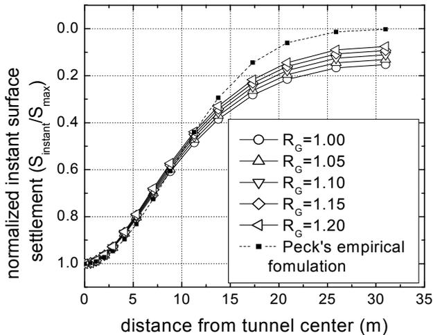
Fig.7 Short-term surface settlement troughs
