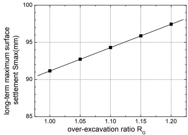
Fig.4 Evolution of long-term surface settlement with over-excavation ratio
