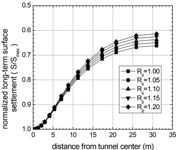
Fig.8 Long-term surface settlement troughs
