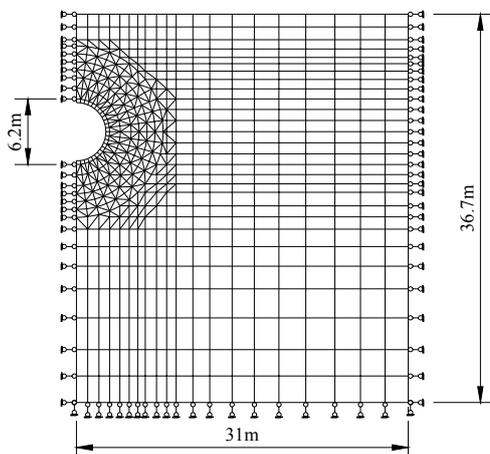
Fig.1 FEM mesh in numerical simulation
