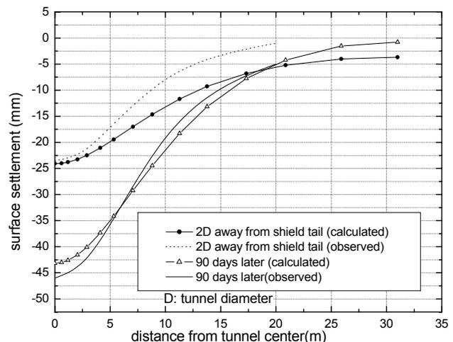
Fig.2 Comparison of calculated and in-situ measured surface settlements
