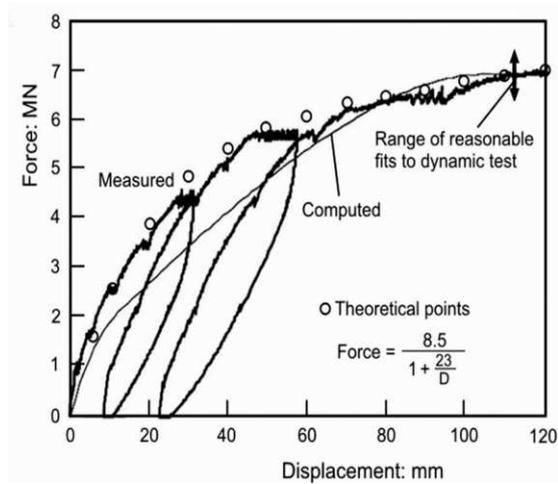
Fig. 13. Comparison of measured, computed and theoretical pile responses (Randolph 2003)
