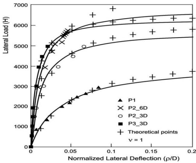
Fig. 8. Load versus normalized lateral deflection. (Experimental data after Ng et al., 2001).
