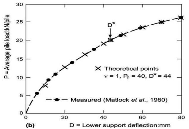
Fig. 6. Load deformation behaviour for (a) a five-pile group and (b) a ten-pile group.
