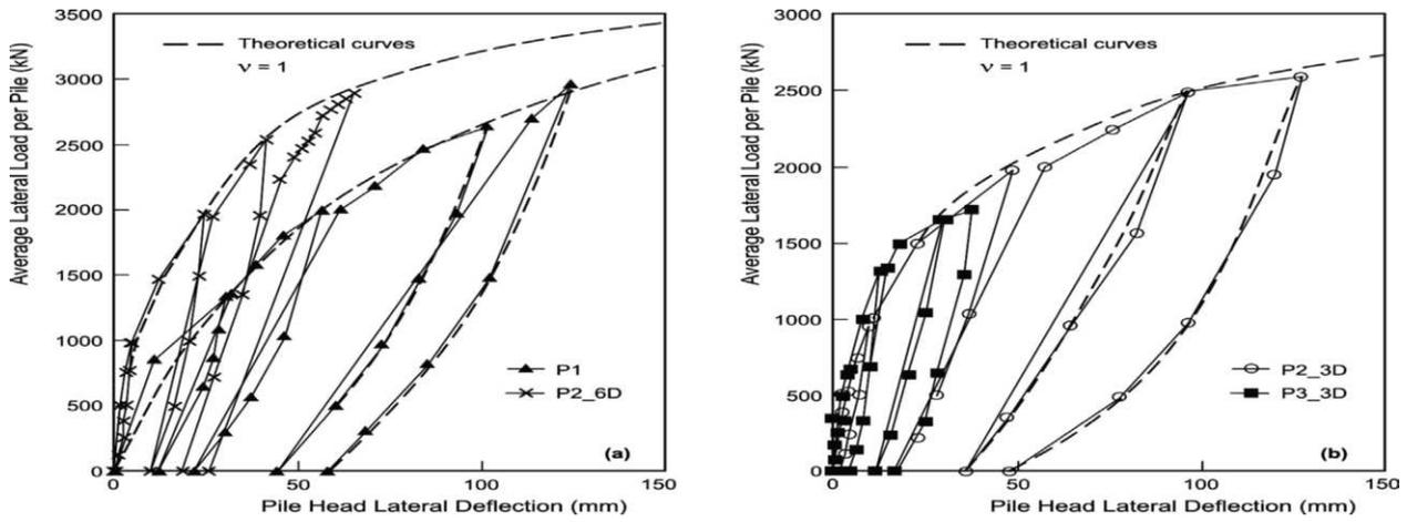
Fig. 7. Load versus deflection: (a) P1 and P2-6D and (b) P2-3D and P3-3D. (Experimental data after Ng et al., 2001).
