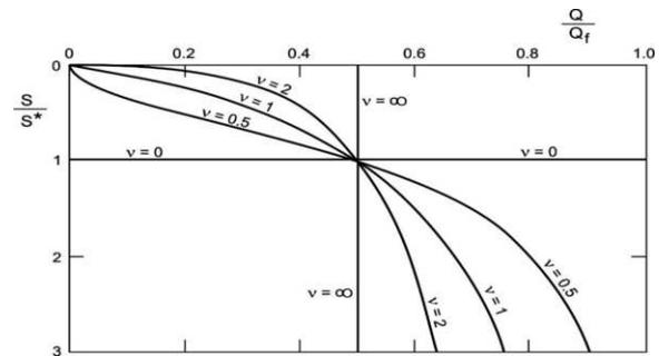
Fig. 3. Graphs of  $Y_s = \frac{Q}{Q_f} = \frac{1}{1 + \left(\frac{S}{S^*}\right)^{-1/v}}$
