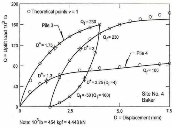
Fig. 4. Uplift load versus displacement for two pile tests in Baker, California, (Konstantinidis et al., 1987).
