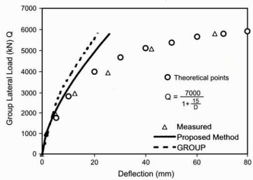
Fig. 15. Comparison of theoretical, predicted and measured lateral displacements for Hong Kong load test (Ooi et al, 2004)
