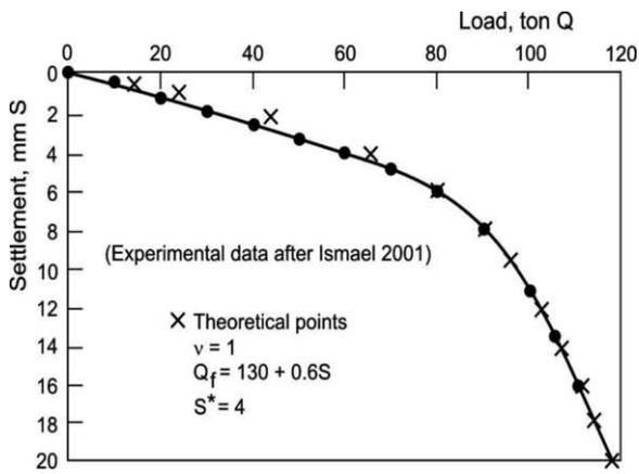
Fig. 12. Load versus settlement for pile group 4.
