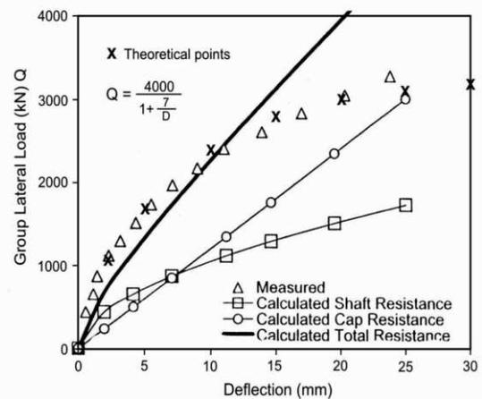
Fig. 16. Comparison of theoretical, predicted and measured lateral displacements of first Las Vegas load test (Ooi et al, 2004).
