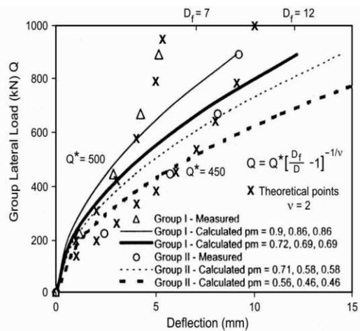
Fig. 17. Comparison of theoretical, predicted and measured lateral displacements for Lewisburg load test (Ooi et al, 2004).
