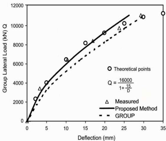
Fig. 14. Comparison of theoretical, predicted and measured lateral displacements for Chaiyi, Taiwan load test (Ooi et al, 2004)
