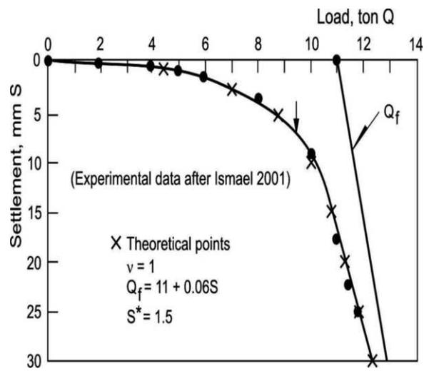
Fig. 10. Load versus settlement for single piles in compression.
