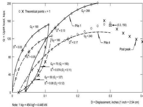
Fig. 5. Uplift load versus displacement for two pile tests in Caliente, Nevada (Konstantinidis et al., 1987).
