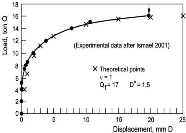
Fig. 9. Load versus displacement for single piles in tension
