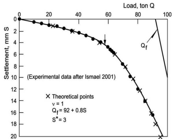
Fig. 11. Load-settlement curve for pile group 3.
