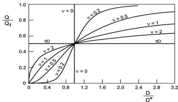
Fig. 1. Graphs of  $Y_s = \frac{Q}{Q_f} = \frac{1}{1 + \left(\frac{D}{D^*}\right)^{-1/v}}$
