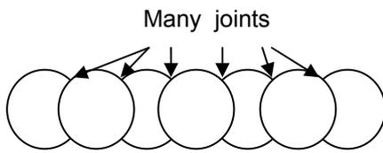
Fig 4: Secant pile wall
