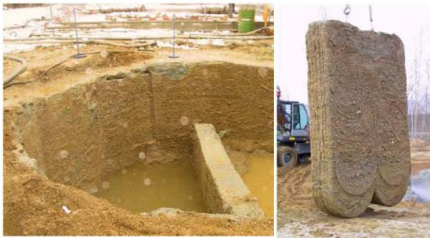
Fig 7: Wall details and exhumed test panel
