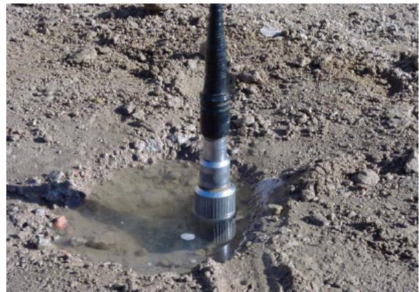
Figure 2: P-S-suspension lowered in the hole filled with water
