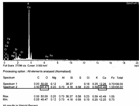
Figure 10. X-ray analysis of CH
