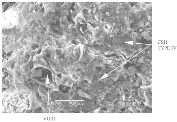
Figure 11. Lab specimens with binder G with amplification factor x550
