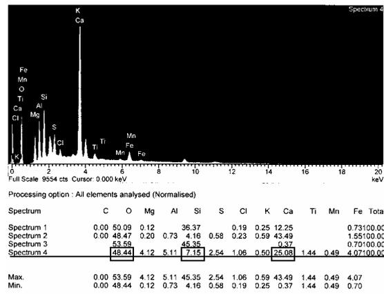
Figure 9. X-ray analysis of CSH gel
