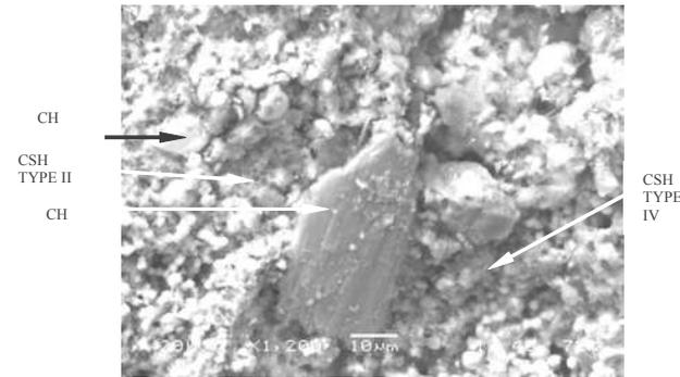
Figure 8. Lab specimens with binder B with amplification factor x1200
