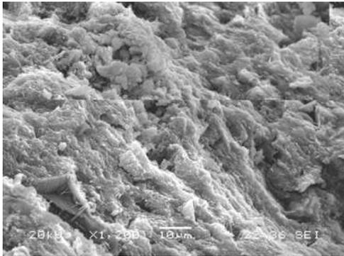
Figure 12. Lab specimen with binder G with amplification factor x1200
