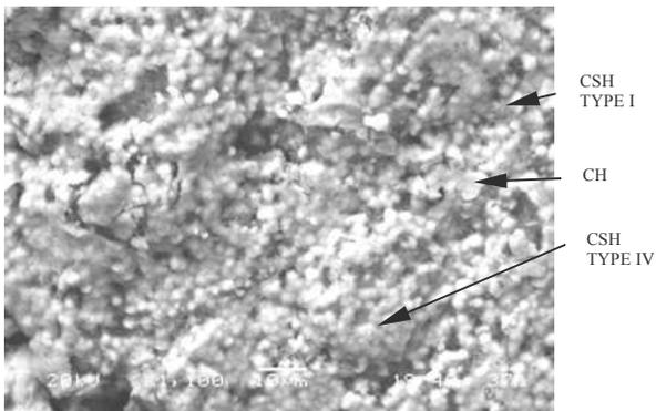
Figure 7. Field specimen with binder B with amplification factor x1100
