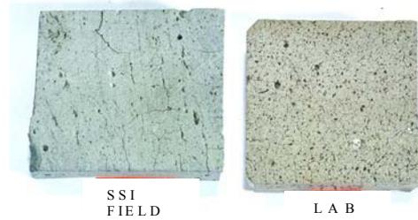
Figure 4. Specimen prepared for SEM investigation from the SSI column and the laboratory treated with binder B
