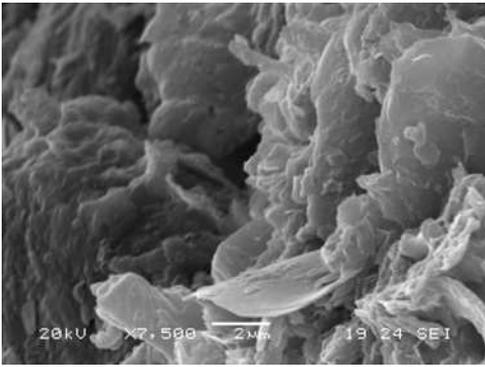
Figure 3. The natural sludge specimen – amplification factor x7500 – illite clay particles are shown here
