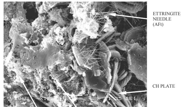
Figure 14. Lab specimen with binder E with amplification factor x1200
