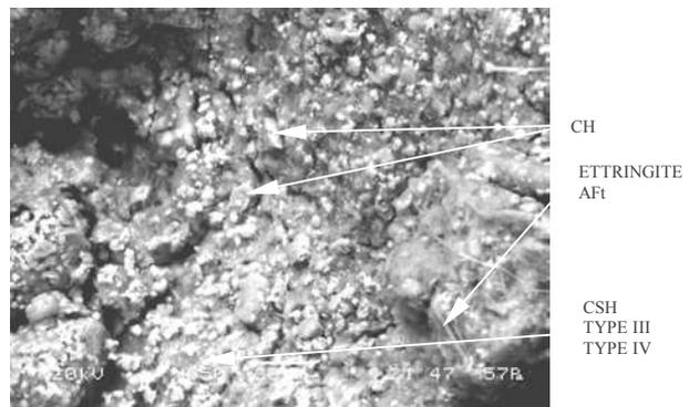
Figure 5. Field specimen with binder B with amplification factor x550
