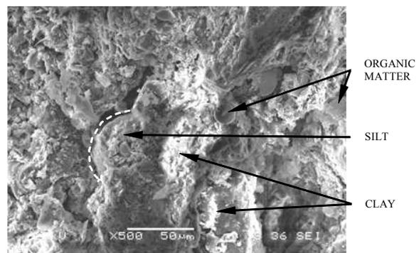
Figure 1. Untreated dredged material specimen – amplification factor x500
