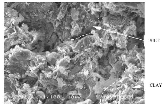
Figure 2. The natural sludge specimen – amplification factor x1100
