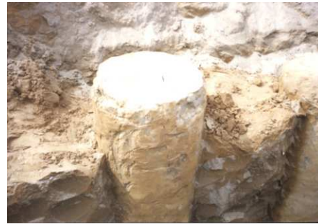
Figure 6. DMM column head before loading test
