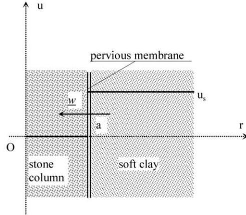
Figure 4. Equivalent membrane at the column-clay interface.
