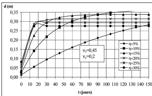
Figure 6. Settlement variation with time of reinforced soil submitted to instantaneous loading ( $E_s=1000\text{kPa}$ ,  $E_c=10000\text{kPa}$ ,  $Q=1000\text{kN}$ ,  $k=10^{-8}\text{ms}^{-1}$ ,  $b=1,7\text{m}$ ,  $H=15\text{m}$ ).
