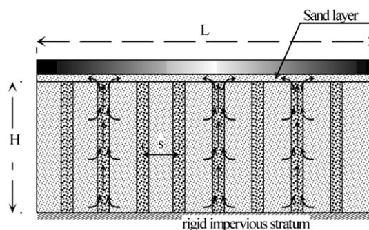
Figure 1. Foundation supported by reinforced soil
