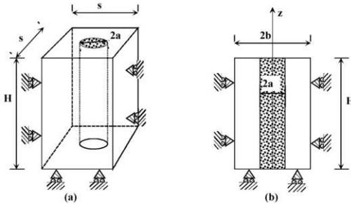
Figure 2. (a) Reinforced unit cell, (b) Auxiliary problem.
