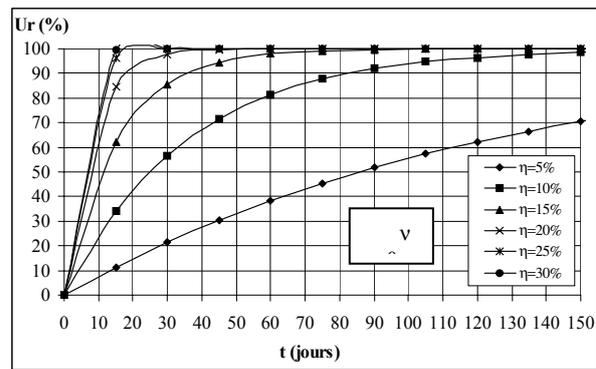
Figure 7. Radial consolidation degree variation as a function of time, of reinforced soil submitted to instantaneous loading ( $E_s=1000\text{kPa}$ ,  $E_c=10000\text{kPa}$ ,  $Q=1000\text{kN}$ ,  $k=10^{-8}\text{ms}^{-1}$ ,  $b=1,7\text{m}$ ,  $H=15\text{m}$ ).
