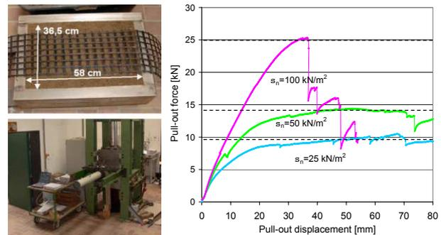
Figure 8. Pull-out resistance test device, dimensions of the shear box and test results (pull-out force versus displacement for different normal stresses)
