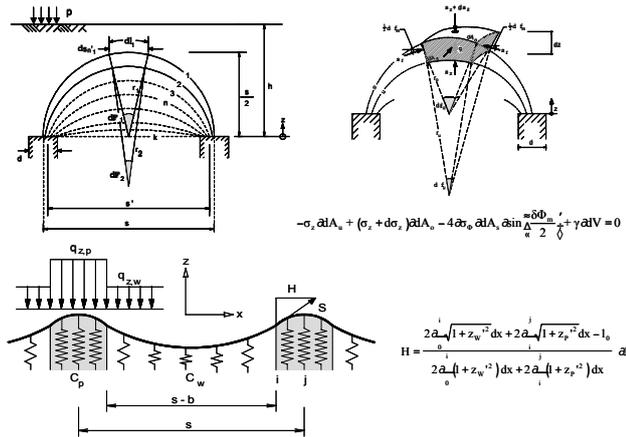
Fig. 9. New soil arching and membrane approach (Zaeske, 2001)
