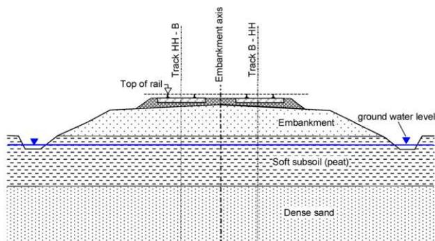
Figure 3. Typical cross-section and soil profile without soil improvement
