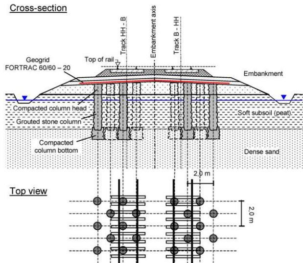
Figure 4. Typical cross-section 1<sup>st</sup> reconstruction stage
