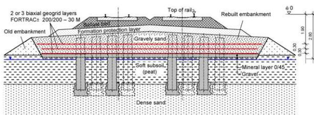
Figure 7. Typical cross-section 2<sup>nd</sup> reconstruction stage
