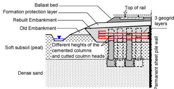
Figure 6. Rebuilt test field, modified double track structure
