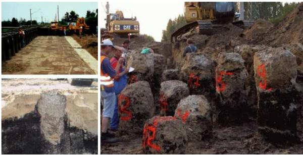
Figure 5. Test field and excavated columns with different heights
