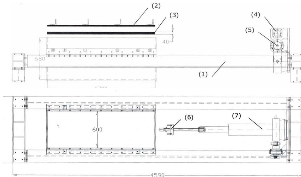
Figure 2 Scheme of pullout test apparatus: 1) frame; 2) steel plate; 3) air bag; 4) electric engine; 5) reducer; 6) load cell; 7) electric jack.
