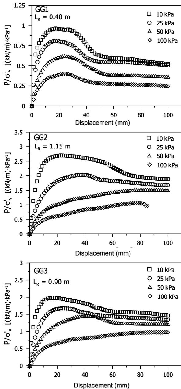
Figure 4. Normalized pullout curves ( $P/\sigma'_v$ ) for the different geogrids.
