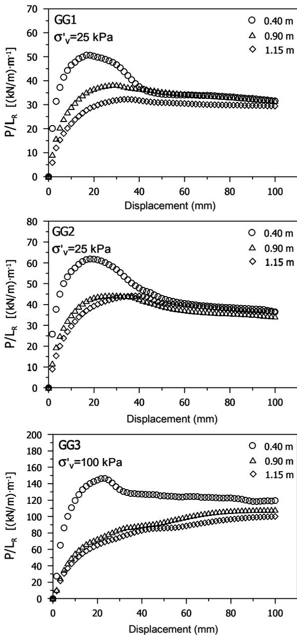
Figure 3. Normalized pullout curves ( $P/L_R$ ) for the different geogrids.
