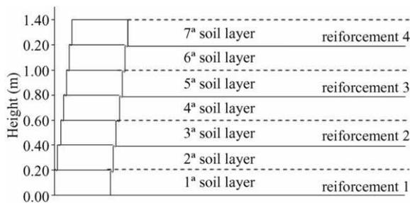
Figure 2 - Construction sequence of the model
