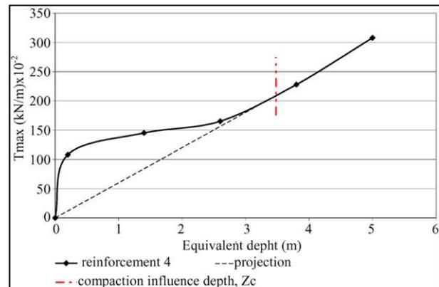
Figure 9 -  $T_{max}$  vs. equivalent depth for the 4<sup>th</sup> reinforcement layer - Wall 2
