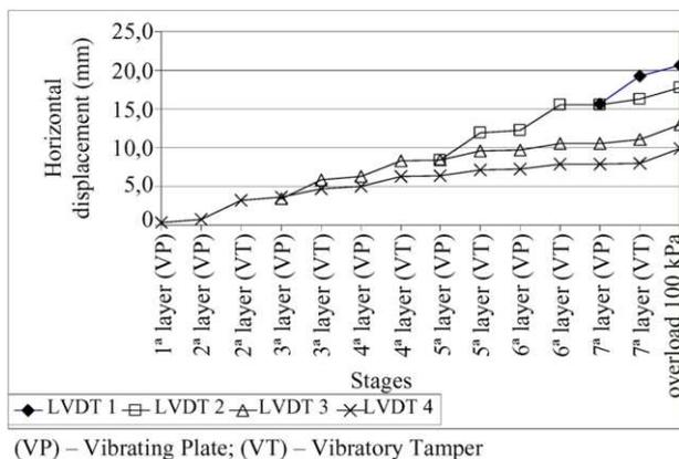
Figure 11 - Accumulated lateral movements of the Wall 2 face at different construction stages and external load application.
