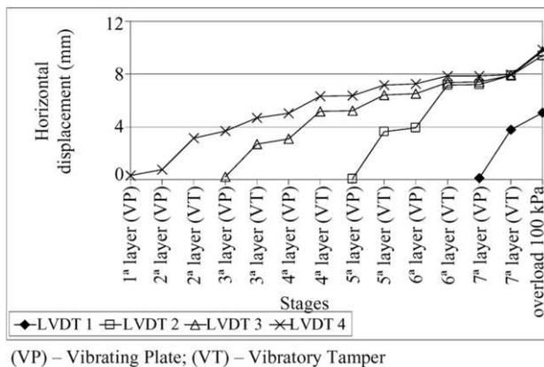
Figure 10 - Measured horizontal displacements of the Wall 2 face at different construction stages and external load application.
