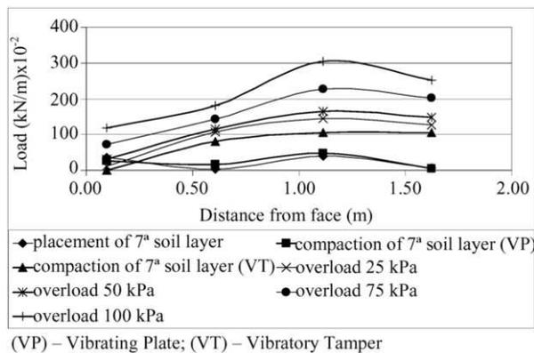
Figure 7 - Measured tension along the reinforcement in the 4<sup>th</sup> reinforcement line - Wall 2
