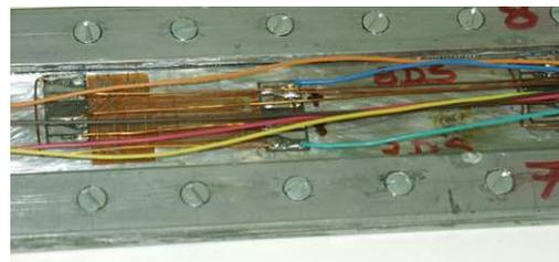
Figure 4 - Load cells without the protection resin.
