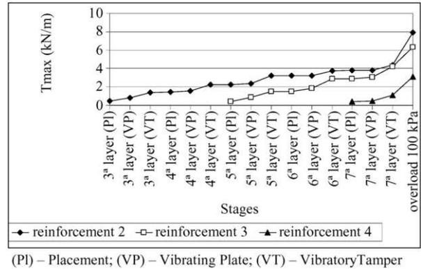
Figure 8 - Measured values of  $T_{max}$  in different layers of reinforcements - Wall 2
