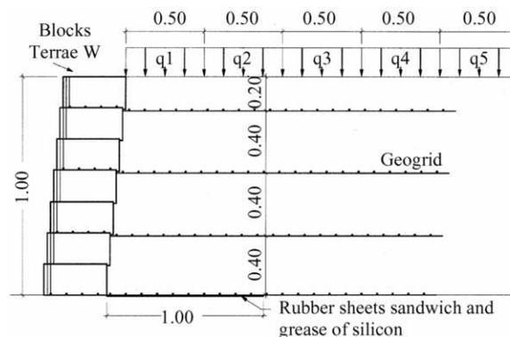
Figure 1 – Model wall section
