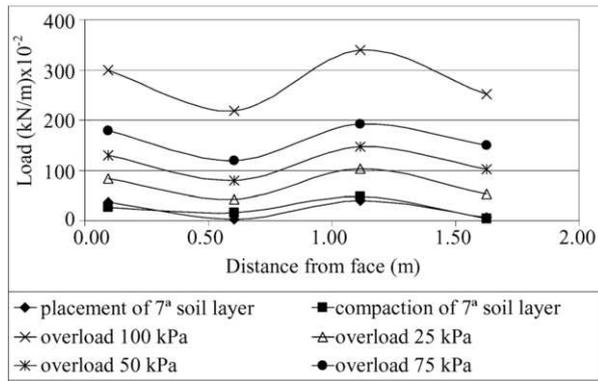
Figure 6 - Measured tension along the reinforcement in the 4<sup>th</sup> reinforcement layer - Wall 1
