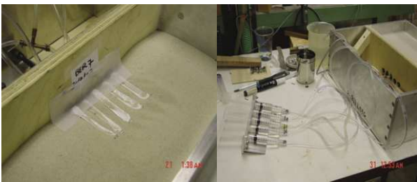
Fig.2 Test setup for simulating expanding tubes in the centrifuge; a) location empty tubes; b) syringe system for expanding tubes.
