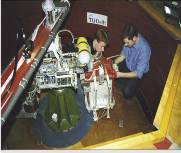
Fig.1 Geotechnical centrifuge of the University of Delft.
