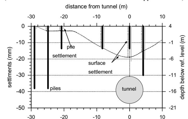
Figure 7. Measured settlement pile v.s. surface settlements, second passage
