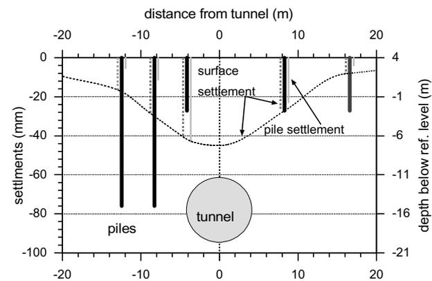
Figure 5. Measured settlement pile v.s. surface settlements, first passage
