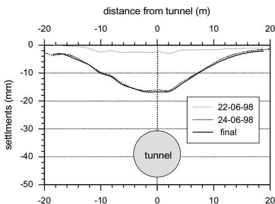
Figure 10. Measured surface settlement. 80% of the surface settlement occurs within two days
