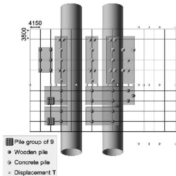
Figure 2. Overview test field with the 2 tunnel tubes. The left tube is drilled first. Numbers give the dimensions of the grid in mm. Gray areas are the loaded areas on the pile foundations. T stands for transducer
