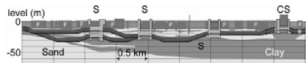
Figure 1. North South line bored tunnel alignment. S are the planned metro stations, CS is the existing train station and F indicates existing pile foundations adjacent to the trace.
