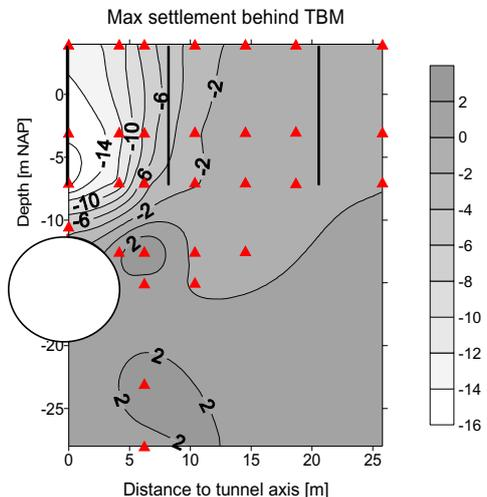
Figure 8. Sub surface settlement contour
