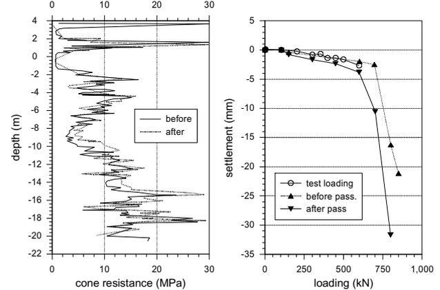
Figure 11. CPT before and after passage TBM, at 3.5 m distance (left). Static pile load tests before and after passage TBM (right).
