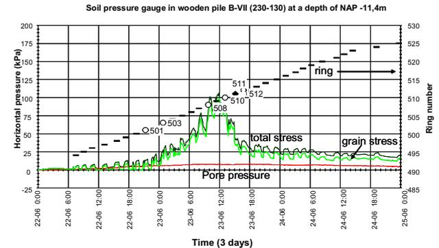
Figure 6. Measured changes in total stress, water pressure and resulting effective stress at pile side during TBM-passage.
