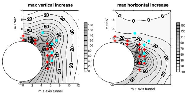
Figure 9. Stress changes after second passage TBM
