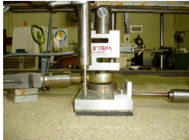
Fig. 2: View of the loading arrangement with the LVDTs in place
