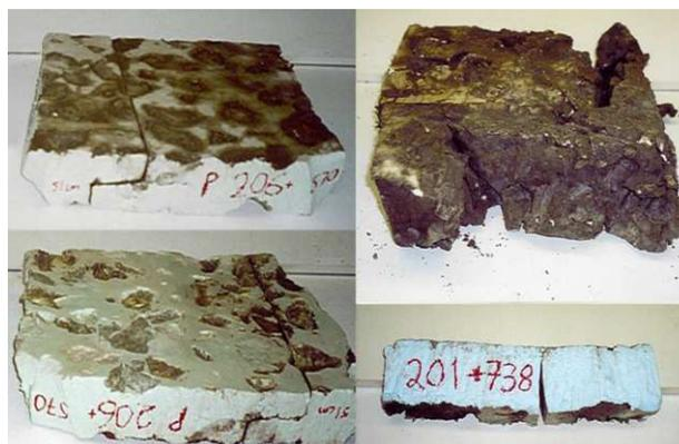
Figure 3. Mechanical damage in XPS frost insulation boards, generally (left), and in the problematic production lot (top right). An example of cracks in the bottom surface of a board, bottom right.
