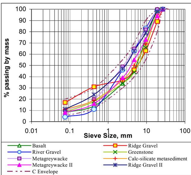
Figure 1: Gradings compared to Specification grading envelope
