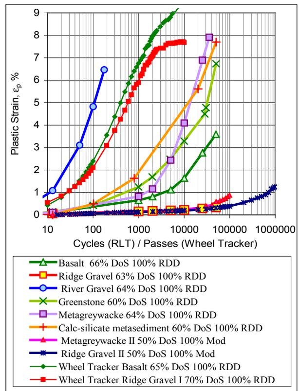
Figure 4: Plastic Strain from RLT and Wheel Tracker
