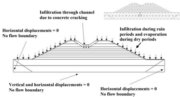
Figure 6. Canal embankment founded on a layer of collapsible natural silts and quadratic triangular elements of the FE discretization.
