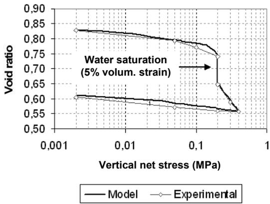
Figure 1. Collapse test on a natural soil from the Segarra-Garrigues canal.
