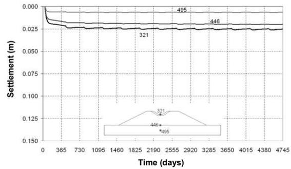
Figure 7. Evolution of settlements of some points due to embankment construction and rainfall action. Embankment founded on natural soils.
