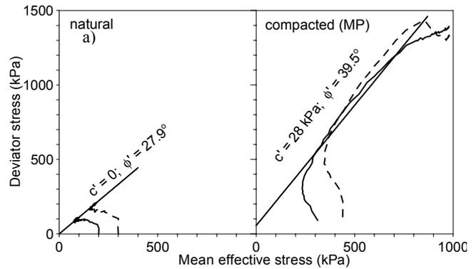
Figure 4. Triaxial CIU tests performed on specimens of natural and compacted silt.
