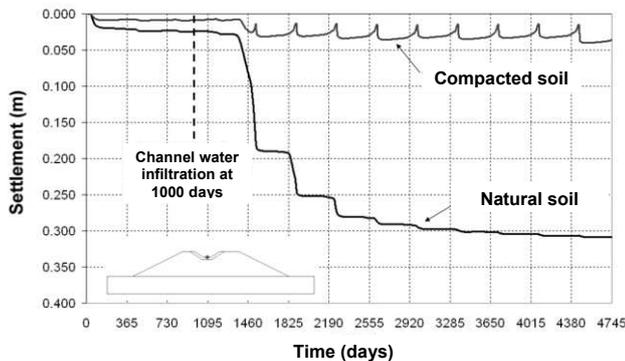
Figure 11. Evolution of settlements of some points due to embankment construction, rainfall action and canal leakage (heavy water losses). Embankment founded on natural soil.
