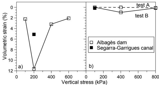
Figure 2. Collapse deformation measured in oedometer tests on a) natural and b) compacted specimens. Segarra-Garrigues and Albagès dam soils.
