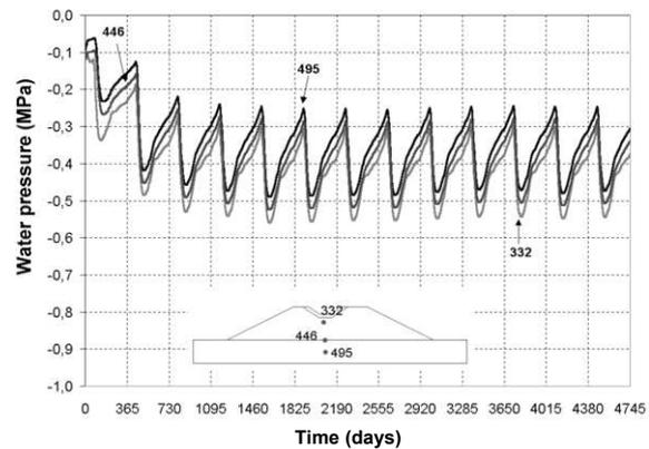
Figure 8. Evolution of pore water pressures of some points due to embankment construction and rainfall action. Embankment founded on natural soils.
