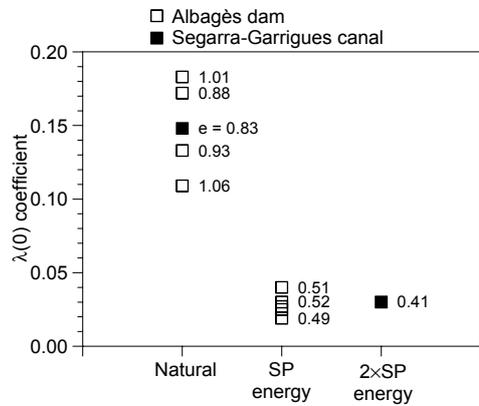
Figure 3.  $\lambda(0)$  coefficient of natural and compacted silt. Void ratio is also annotated.
