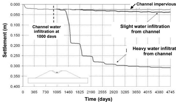
Figure 10. Evolution of settlements of some points due to embankment construction, rainfall action and canal leakage (slight water losses). Embankment founded on natural soil.
