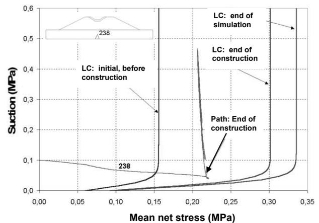
Figure 9. Stress paths of some points during embankment construction and rainfall action. Embankment founded on natural soils.
