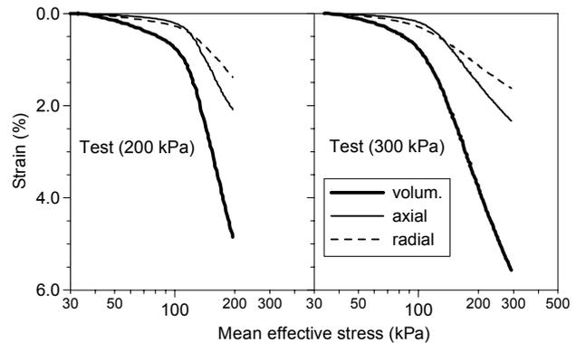
Figure 5. Isotropic compression stage of two specimens of silt in natural state.
