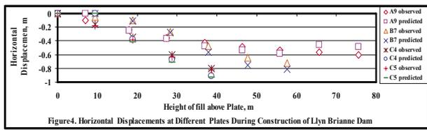
Figure 4. Horizontal Displacements at Different Plates During Construction of Llyn Brienne Dam
