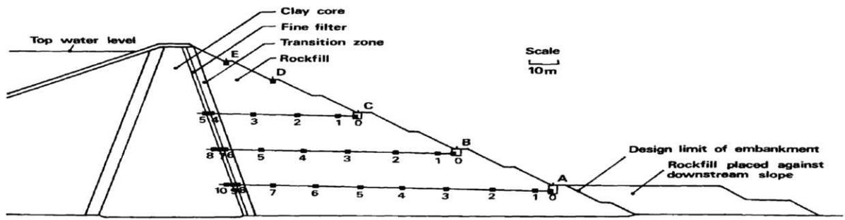
Figure 1. Cross Section of Llyn Brianne Dam Showing Position of Plate Gauges (after Penman and Charles, 1972a).
