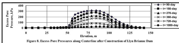
Figure 8. Excess Pore Pressures along Centerline after Construction of Llyn Brienne Dam
