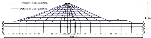
Figure 3. The Deformed Shape of Llyn Brienne Dam During Construction.
