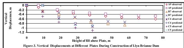
Figure 3. Vertical Displacements at Different Plates During Construction of Llyn Brianne Dam
