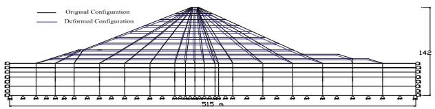
Figure 4. The Deformed Shape of Llyn Brienne Dam after Construction.
