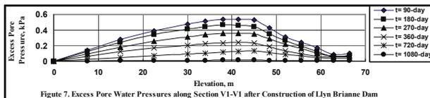
Figure 7. Excess Pore Water Pressures along Section V1-V1 after Construction of Llyn Brienne Dam
