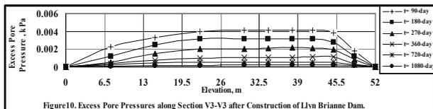
Figure 10. Excess Pore Pressures along Section V3-V3 after Construction of Llyn Brienne Dam.
