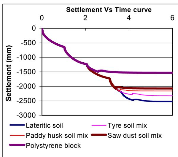
Figure 4. Construction results of 3m embankments over 8m depth peaty clay - process.
