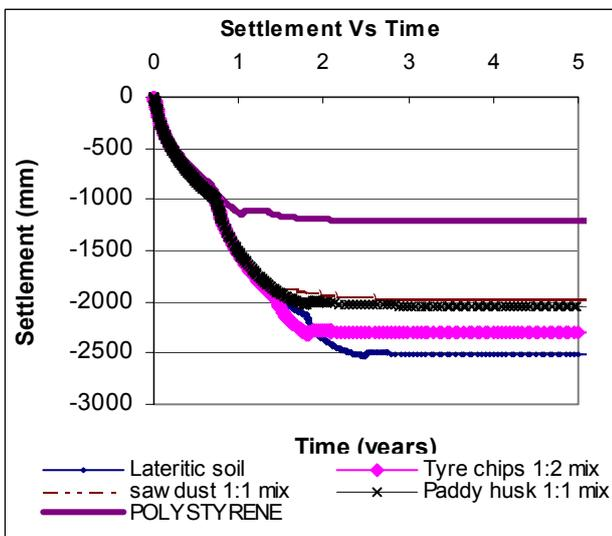
Figure 6. Construction result of 3m embankments over 8m depth peaty clay with 2m crust.
