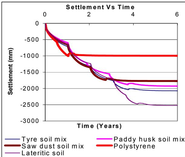
Figure 5 Construction results of 3m embankments over 8m depth peaty clay –process2.
