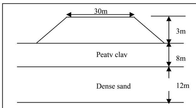
Figure 1. The soil profile and the embankment geometry
