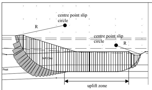
Figure 3. Calculated effective vertical stresses of the Uplift Van model
