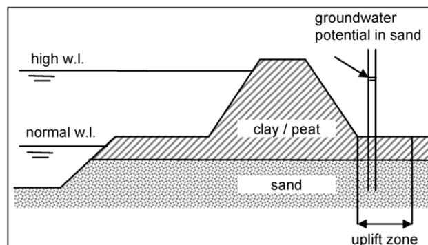
Figure 2. Typical dike section for Hollandprofile
