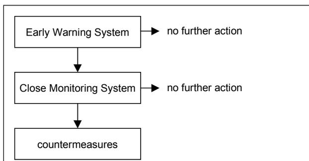
Figure 1. Scheme of the proposed observational method for dike management
