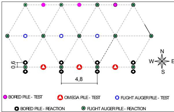
Figure 2. Pile location on the Experimental Field.
