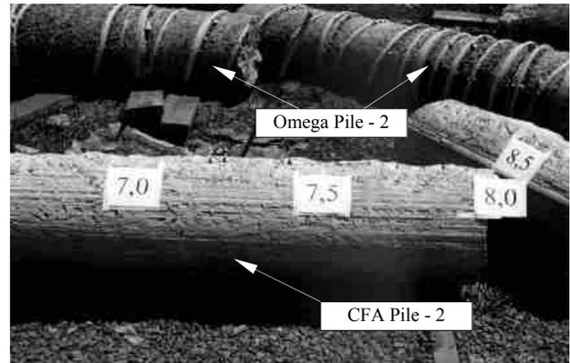
Photo 1: shape of the Omega 2 shaft as compared to CFA 2 shaft
