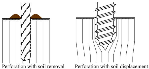
Figure 1. Different forms of excavation (Van Impe, 1988).
