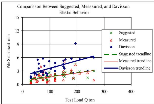
Figure 3. Elastic behavior for test load one and half the working load.
