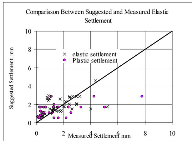
Figure 6. Measured and suggested elastic and plastic pile load settlement in case the test load is one and half the working load.
