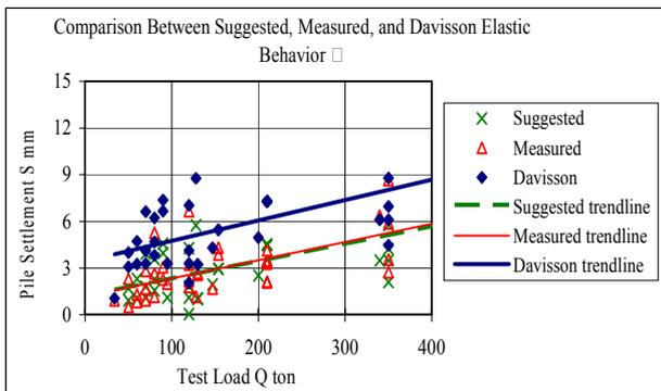
Figure 5. Elastic behavior for test loads twice the working load.
