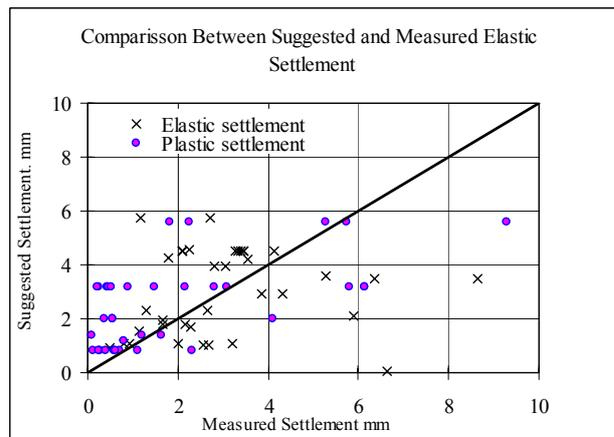
Figure 7. Measured and suggested elastic and plastic pile load settlement in case the test load is twice the working load.
