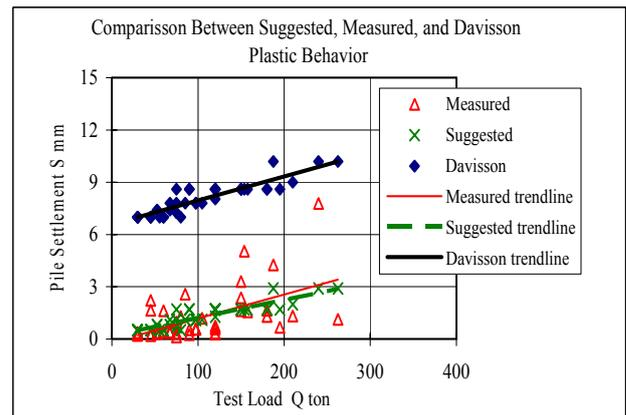
Figure 2. Plastic behavior for test load one and half the working load.
