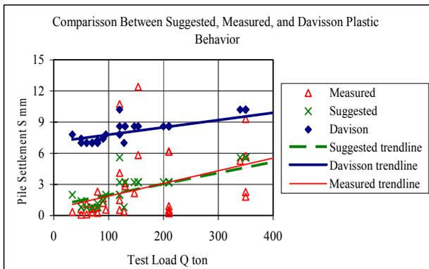
Figure 4. Plastic behavior for test load twice the working load.
