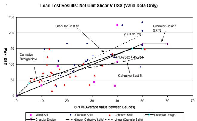
Figure 3. Graphical presentation of processed test pile results from C270
