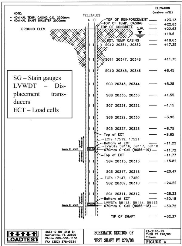
Figure 2 Typical test pile arrangement
