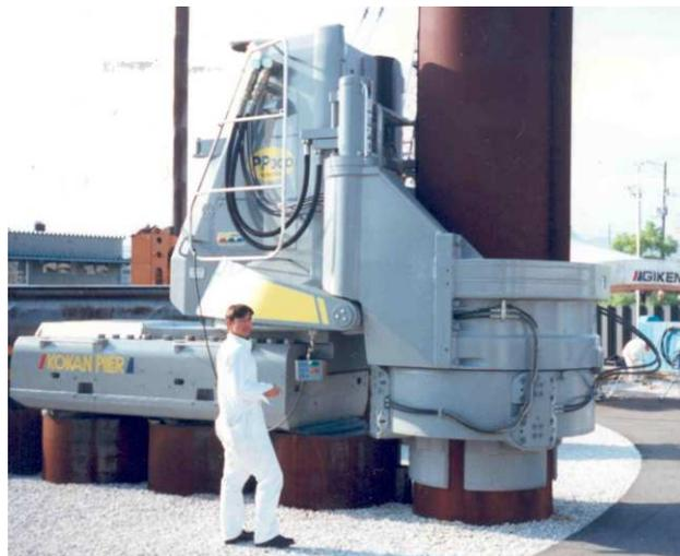
Figure 1. A ‘press-in’ piling machine for installing large tubular piles
