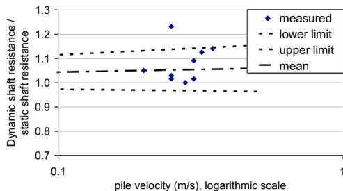
Figure 8 Loading rate local shaft resistance
