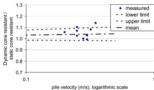
Figure 7 Loading rate tip resistance
