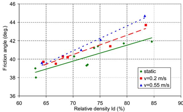
Figure 5 Measured friction angle – relative density relation
