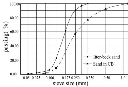
Figure 2 Grain size distribution curve
