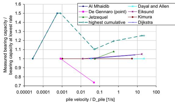
Figure 1 Influence of loading velocity on bearing capacity, normalized arbitrarily on the lowest velocity/pile diameter
