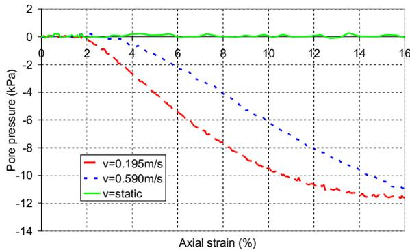
Figure 4 Excess pore pressure on axial strain
