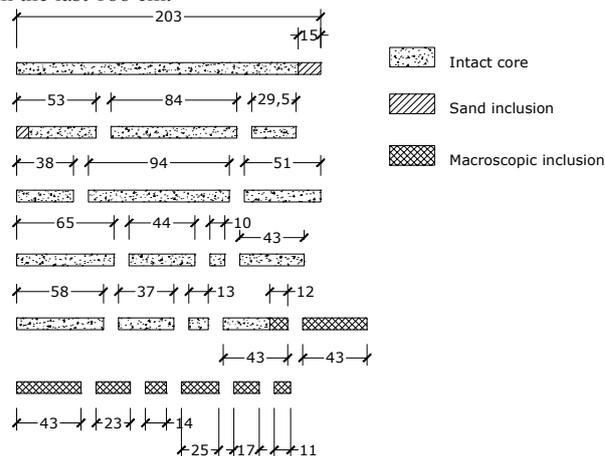
Figure 10. The axial profile of the concrete, bored through pile nr. 270, bears evidence of a total length of 10.41 m and of the definite presence of rubble along the last 1.88 meters.
