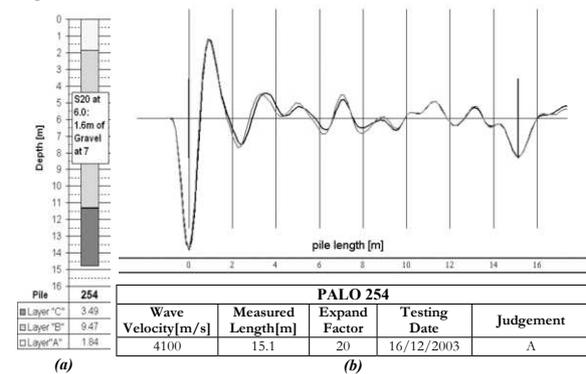
Figure 6. Revised result for pile nr. 254, keeping into account of the anomaly represented by a 1.6 m thick gravel pocket (inset in a) found at 7 meters from the GL.
