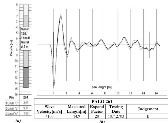
Figure 7. Revised result for pile nr. 261, due to the same gravel lens as said in Fig. 6, found in the nearby borehole nr. 20 at 7 meters from the GL.
