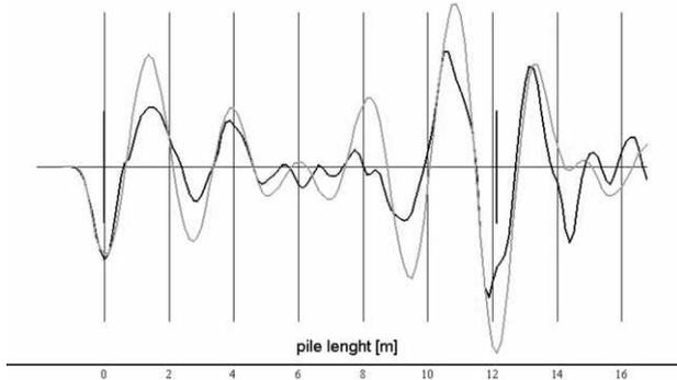
Figure 4. Pile 53 (BD): erratic output due to superficial concrete discontinuities; in grey one of the 30 blows, in black the averaged signal.
