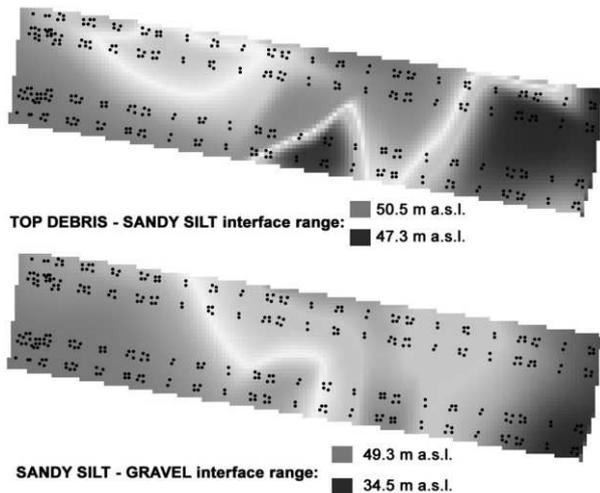
Figure 2. The interface interpolations for the three layers', within the pile group.
