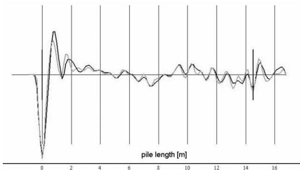
Figure 5. Pile 53 (AD): output signal through intact concrete.
