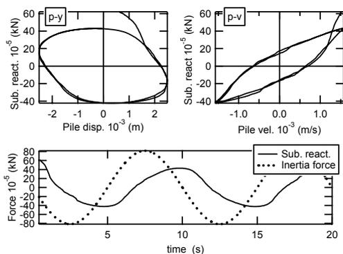
Figure 7. P-y and p-v relations and time histories of subgrade reaction and inertia force (case c-m1)
