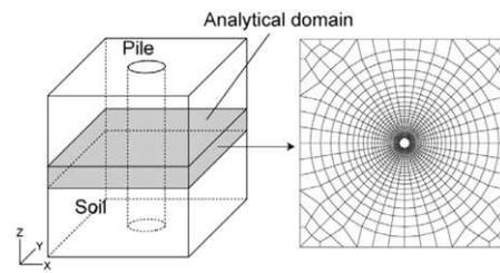
Figure 2. Concept of the numerical model
