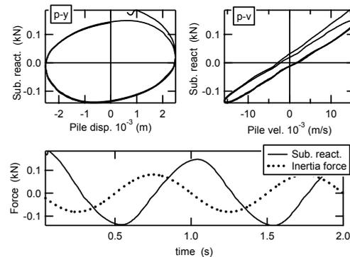
Figure 4. P-y and p-v relations and time histories of subgrade reaction and inertia force (case c-h2)
