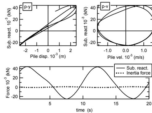
Figure 3. P-y and p-v relations and time histories of subgrade reaction and inertia force (case c-h1)
