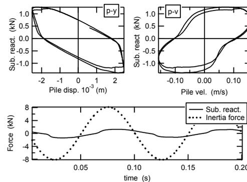
Figure 5. P-y and p-v relations and time histories of subgrade reaction and inertia force (case c-h3)
