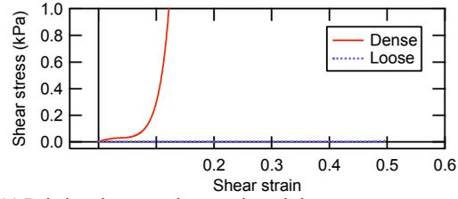
(a) Relations between shear strain and shear stress
