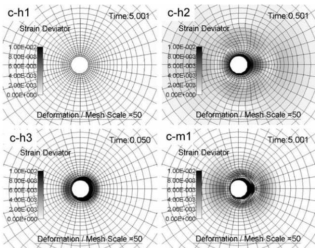
Figure 6. Deformed configuration and distribution of strain deviator (case c-h1, c-h2, c-h3 and c-m1)
