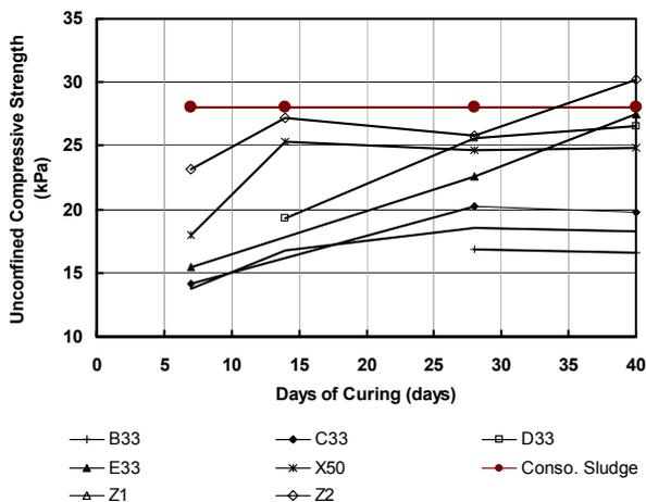
Figure 2 Results of unconfined compression test results
