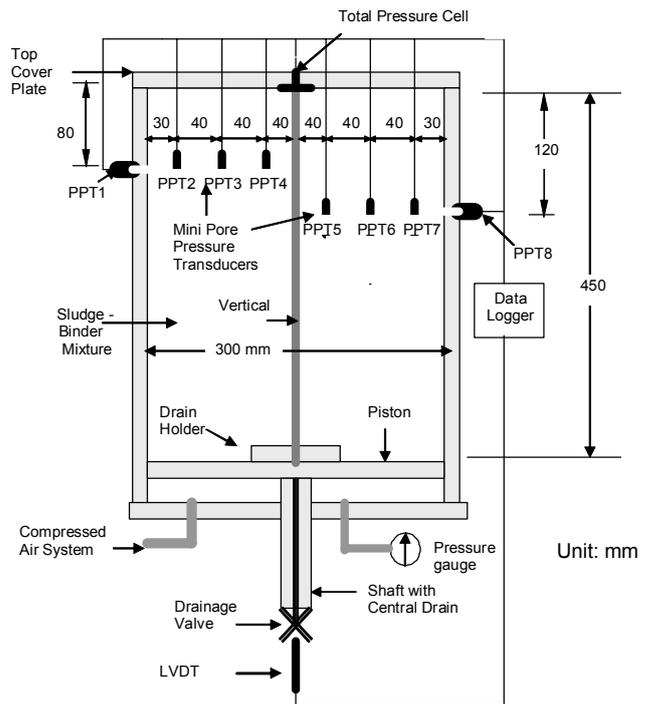
Figure 3 Schematic arrangement of consolidation test
