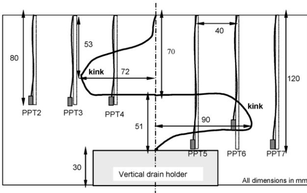
Figure 7 Deformation profile of vertical drain at the end of the test
