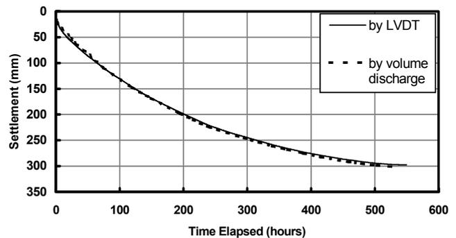
Figure 4 Settlement versus time curve measured during consolidation
