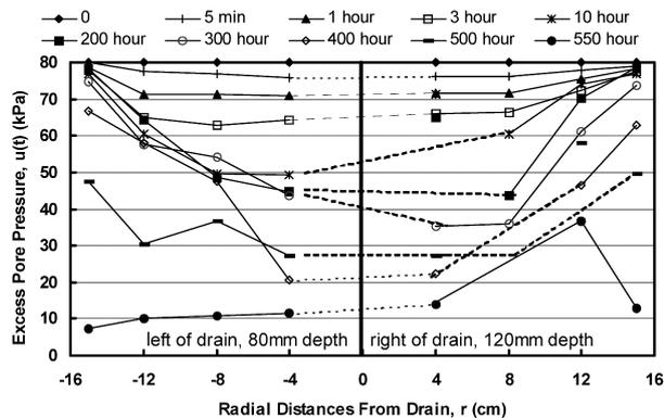
Figure 6 Isochrones of excess pore pressure distribution along the radial distance from the drain at different time intervals.
