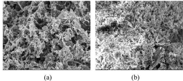
Figure 8 Microstructure of (a) pure sludge and (b) treated sludge
