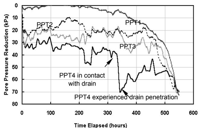
Figure 5 Pore water pressure dissipation versus time curve measured during consolidation
