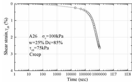
Figure 10. Results of creep shear tests (incinerated ash).
