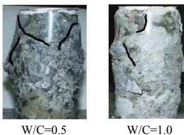
Figure 13. Cement-mixed Specimens after shear testing.
