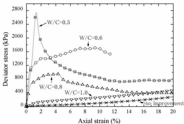
Figure 12. Stress-strain relationship of cement-mixed incombustible waste.
