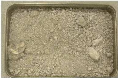
Figure 3. Incinerated ash from Tokyo's Waste Deposit.
