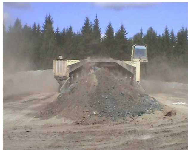
Figure 4: Stack mixer mixing fibre-ash (Kukkia Circlet, Pilot 2003)
