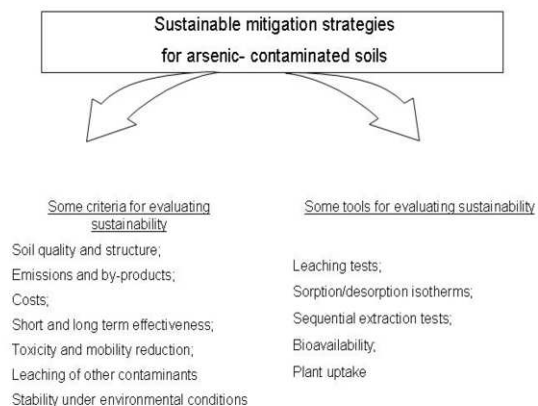
Figure 5. Some of the criteria and tools for evaluating technologies and protocols for environmental management of arsenic-contaminated soils
