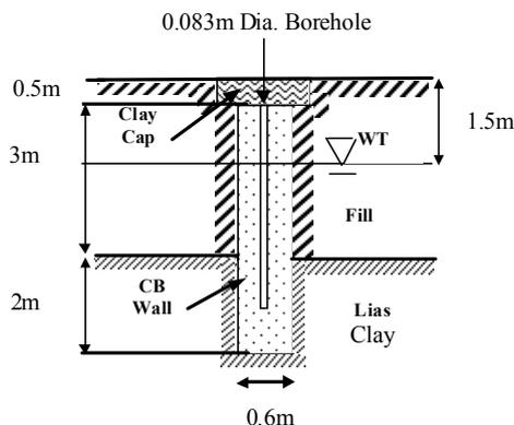
Fig. 3 Typical cross section
