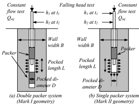
Fig. 1 Packer test configurations
