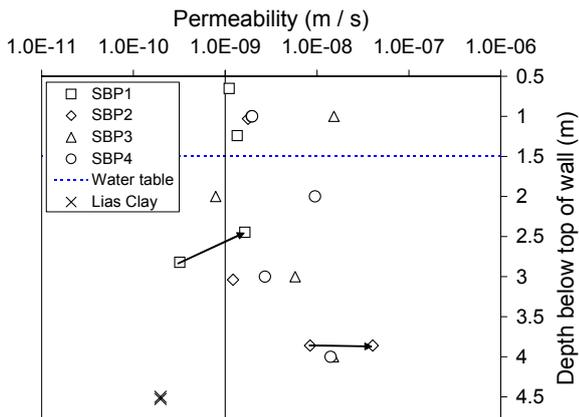
Fig. 5 Permeability values from SBP testing
