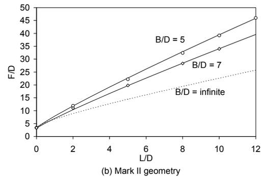
Fig. 2 Normalised shape factor  $F/D$  as a function of  $L/D$  and  $B/D$
