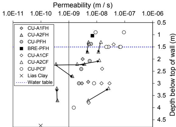
Fig. 4 Permeability values from packer system testing
